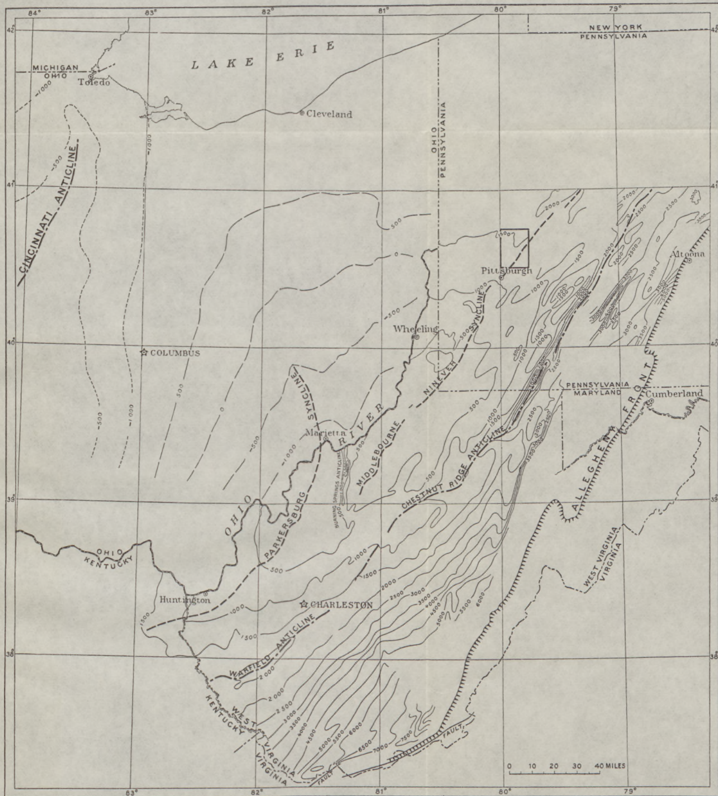
CONTOUR MAP SHOWING GENERALIZED GEOLOGIC STRUCTURE OF PART OF THE PITTSBURGH-HUNTINGTON BASIN
