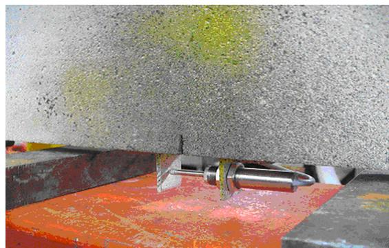
Figure 3.12. Measurement instrumentation: (a) digital camera Canon EOS–1Ds Mark II in front of a small size beam, (b) induction displacement gauge at the beam covered with the black–yellow pattern inside the image area of interest
