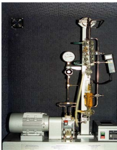
Fot. 1 Pump-injector rig
