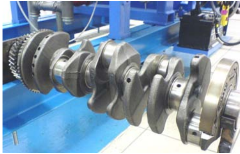
Fig. 1. General view of engine crankshaft, inertial vibration damper on the right
