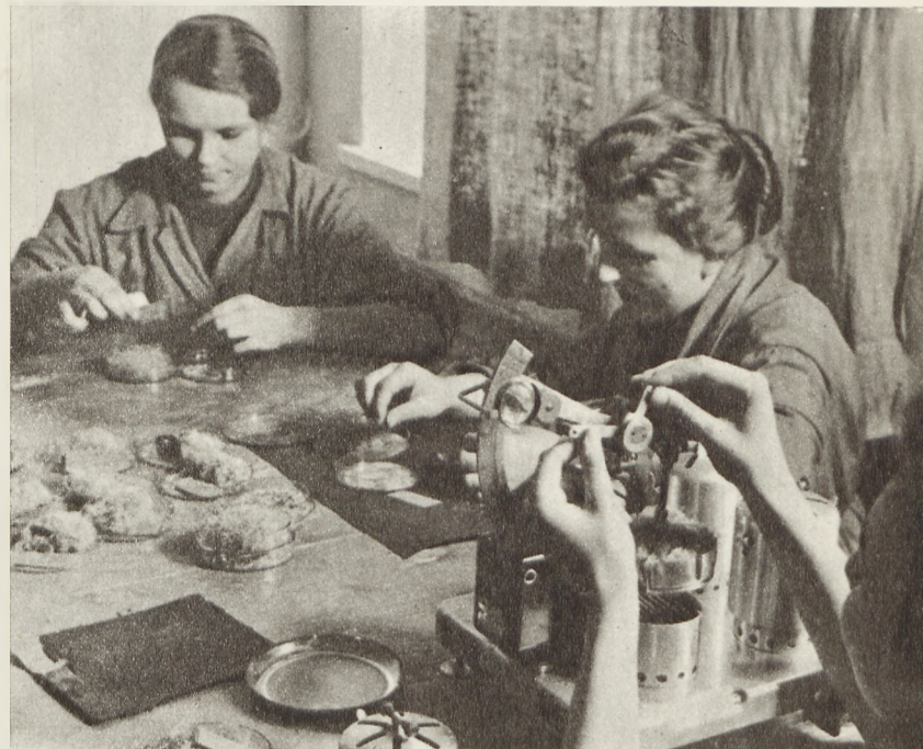
Standards routine for flax tow: moisture test and examination for shives
