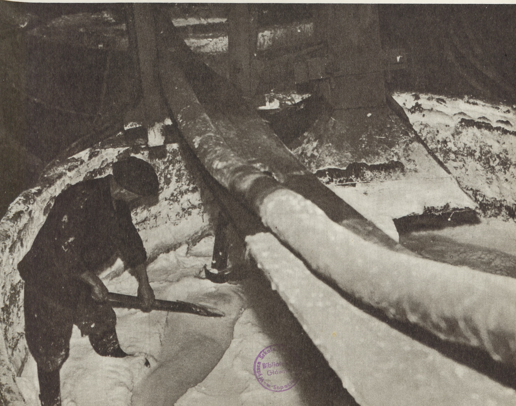
Attending to the sal ammoniac crystallisation process
