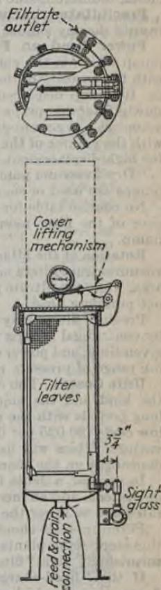
Fig. 24.—Oliver pressure filter.
