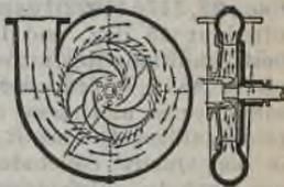
FIG. 5.—Centrifugal pump.
