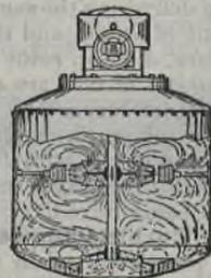
Fig. 28.—Turbine mixer with stationary deflecting blades.
