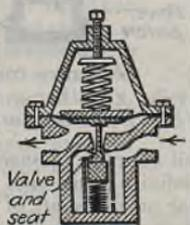
FIG. 30.—Spring-operated pressure reducing valve.
