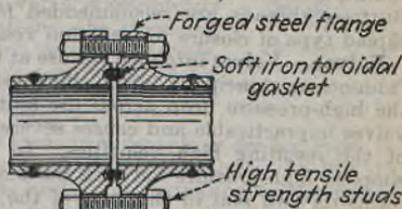
FIG. 10.—Ring joint for large tubes.
