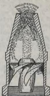
FIG. 4.—Solid-cone nozzle. (Courtesy of The Spray Engineering Co.)
