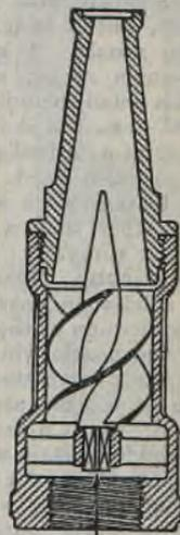
FIG. 3.—A large hollow-cone nozzle. (Courtesy of Schutte and Koerting Co.)
