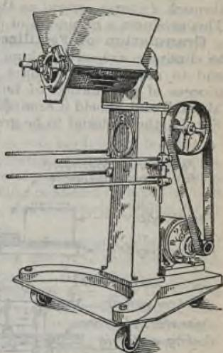
FIG. 10.—Oscillating granulator, assembly. (Courtesy of F. J. Stokes Machine Co.)
