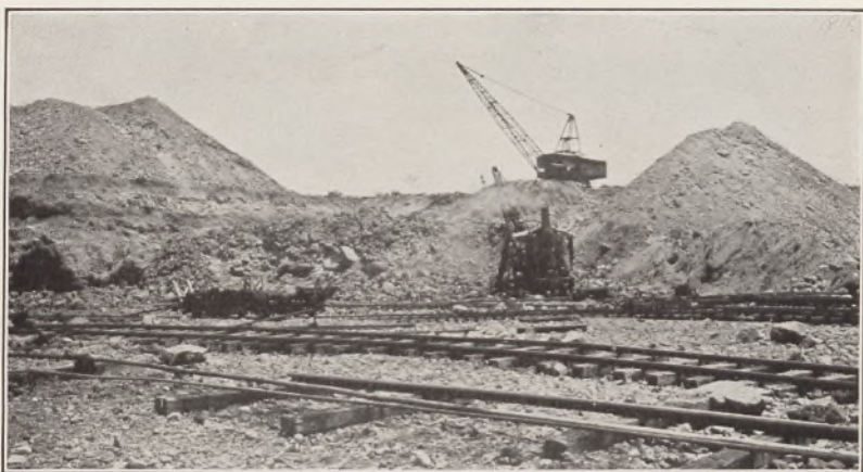
A. QUARRY IN POROUS ANACACHO LIMESTONE IMPREGNATED WITH ASPHALT, SOUTHEAST OF CLINE, TEX.
