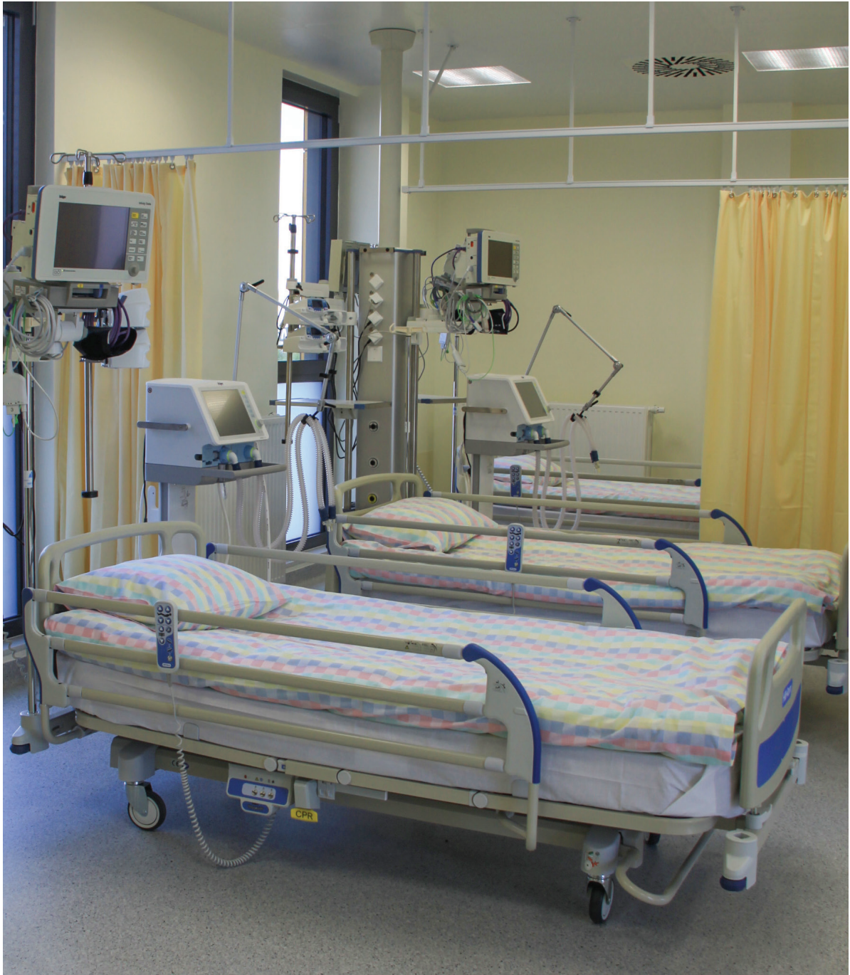
Photograph 6.2.4.4 The curtains between patient stations (an example of a conflict between the need for privacy and epidemiological safety; curtains can become hospital-acquired infection sources); photographed by the Author, 2019
