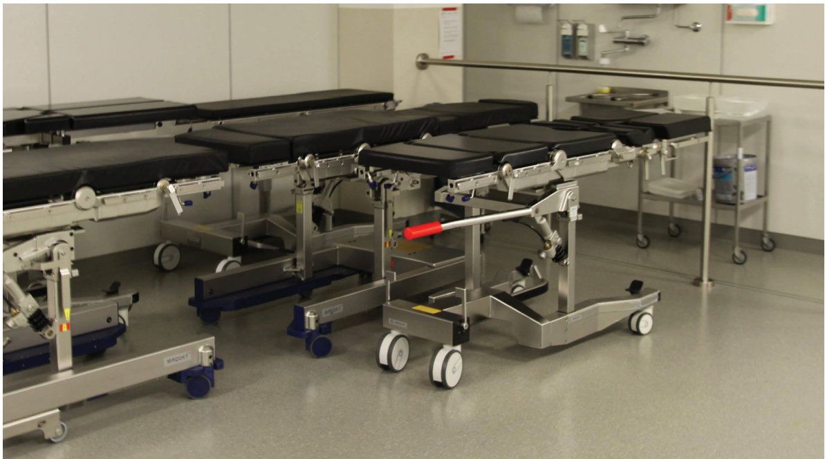
Photograph 5.4.2 A decontamination station for mobile operating tables in the general circulation in an operating suite; photographed by the Author 2016
