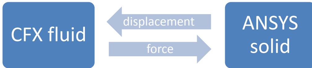
Figure 4.6. Structural coupling information exchange
