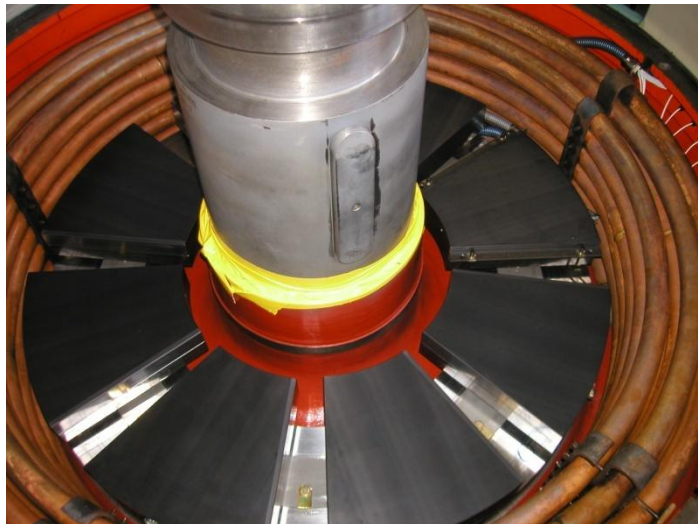
Figure 2.20. Internal water cooler in the bearing housing (ALSTOM Hydro)
