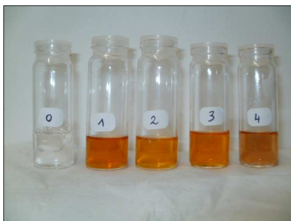
Figure III-33. Characteristic orange colour of hydroxamate 15-18 complexes with \text{Fe}^{3+} , samples 1-4 and 0 correspond to the ligands 15-18 and to the blank experiment without the ligand, respectively
