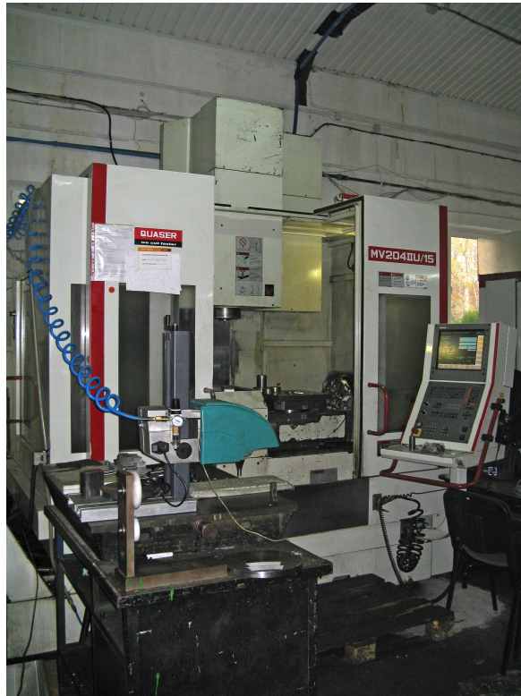
Rys. 38. Frezarka Quaser MV204IU/15
