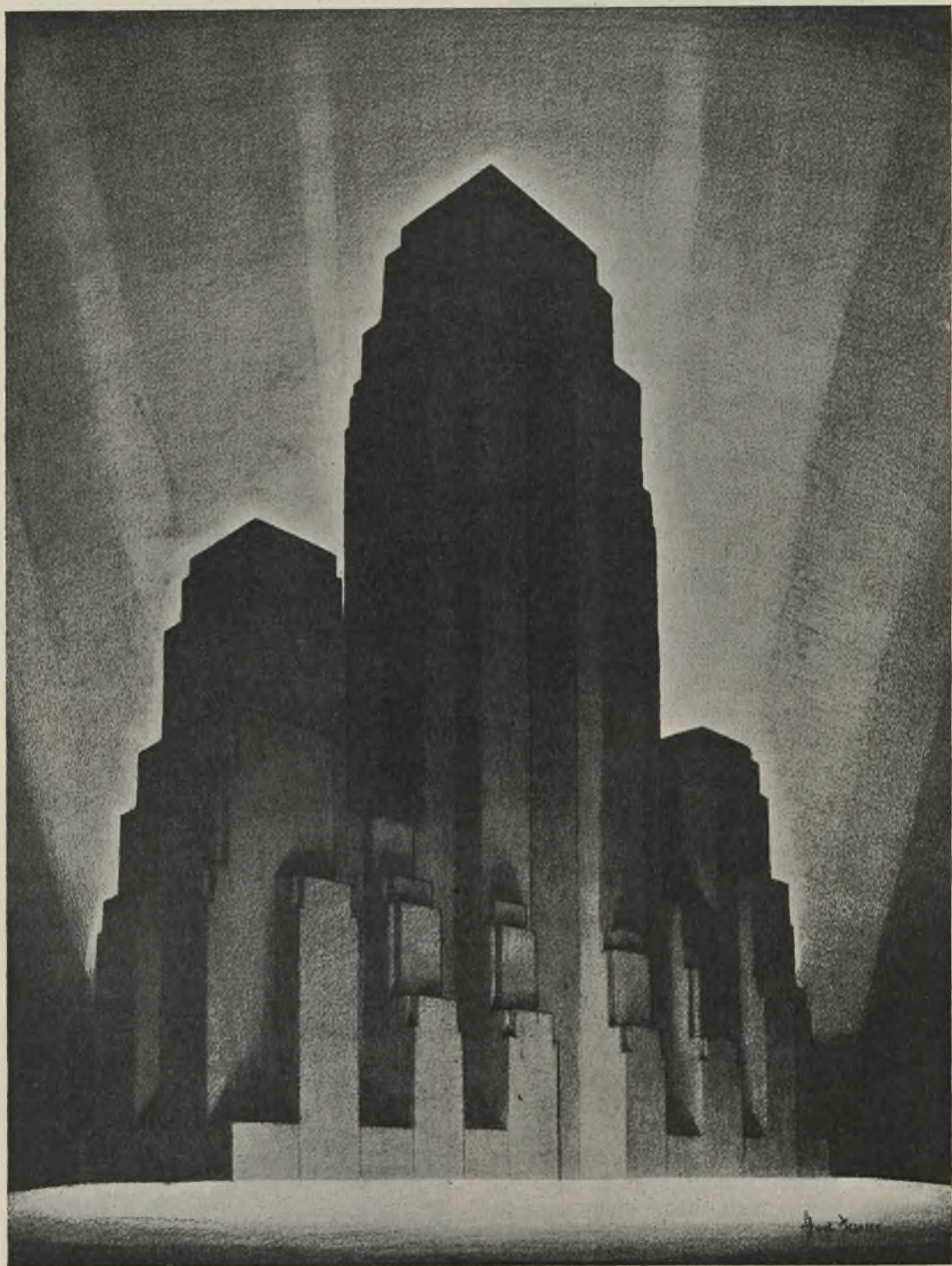
"THE ENVELOPE," FOURTH STAGE (THE PRACTICAL SOLUTION OF THE MASS SHOWN OPPOSITE). DRAWN BY HUGH FERRISS FROM THE PLANS OF HARVEY WILEY CORBETT
