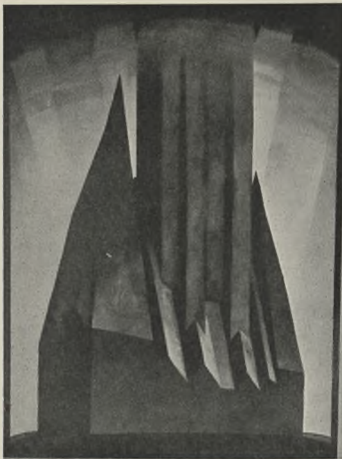
"THE ENVELOPE," FIRST STAGE (MAXIMUM MASS PERMITTED BY THE NEW YORK ZONING LAW ON A FULL CITY BLOCK). DRAWN BY HUGH FERRISS FROM THE PLANS OF HARVEY WILEY CORBETT
