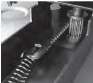
Fig. 11.8. Rack and pinion gears from a household scale
