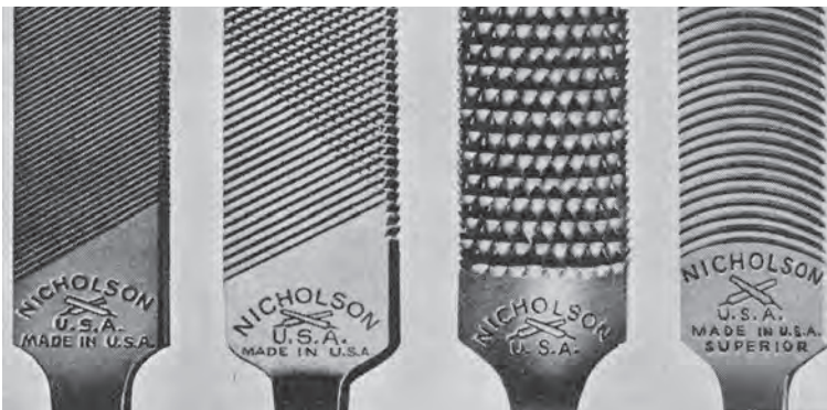
Fig. 2.3. Files. A – single-cut, B – double-cut, C – rasp, D – curved-tooth
