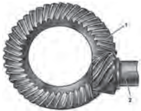
Fig. 11.6. Hypoid bevel gears in a car differential: 1 – ring gear, 2 – pinion gear
