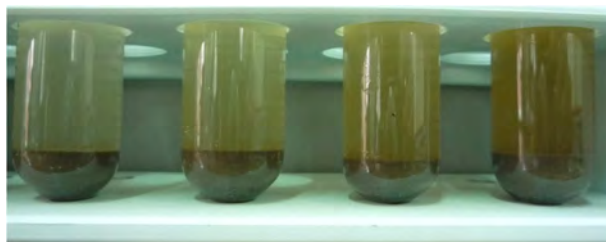
Figure 46. Lindum soil in solution containing increasing concentration of [OMIM][Cl]
