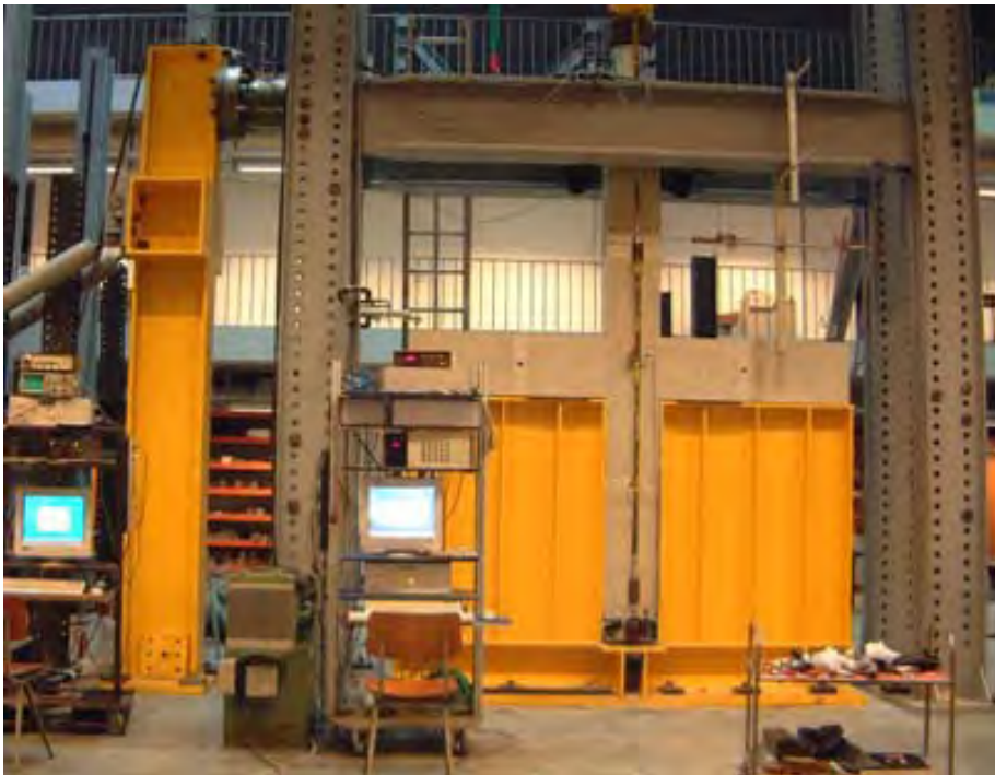
Fig. 2.10: The test setup reproducing a 'weak beam - strong column' configuration (Plumier et al. 2005)
