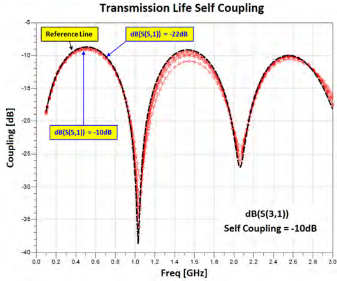
Figure 4.11: The simulation results for shifted coupler configuration. The dependency of the transmission line self coupling and the coupler's branch coupling factor for M_L = -10\text{dB}
