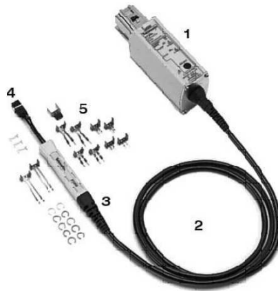
Figure 2.22: Modern oscilloscope probe. (1) a circuit that controls the probe and communicates with oscilloscope, (2) 50\Omega coaxial cable, (3) a probe amplifier which acquires a signal from the device under test to the buffer which drives 50\Omega line, (4) attachment for the two small coaxial cables to differential signal measurement, (5) the probe tip which is the point of contact between the circuit under test and the probe [97]
