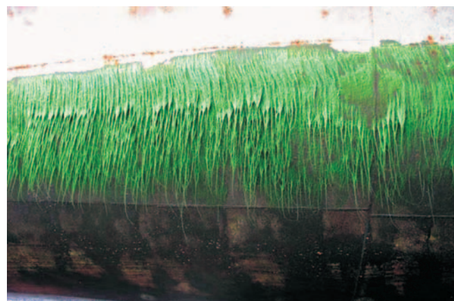
Fig. 4. Algae fouling the ship hull .
