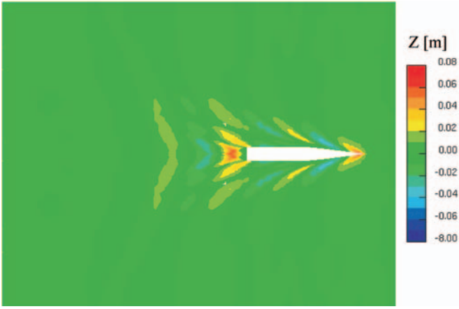
Fig. 16. Wave contour at Froude number Fn = 0.3 .
