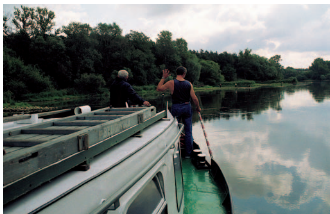
Photo 4. (J. Kulczyk, R. Werszko) A shoal patch of about 1-1.2 m water depth and many erratic boulders resting on the river bed section of some kilometers in length and located close to Puszczykowo upon the Warta. A crew member is heaving the lead and showing its result to the ship master .
