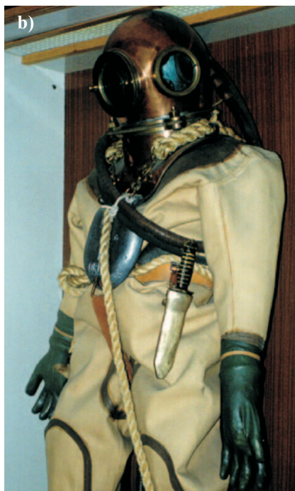
Photo 1b. The diving equipment with helmet UWS-50m (the own photography)
