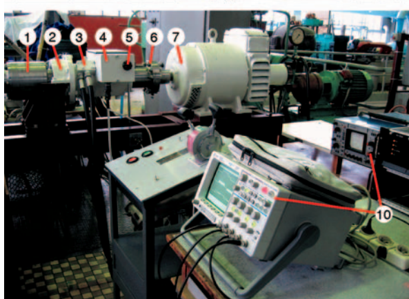
Fig. 3. The laboratory stand for testing the CP propeller servomechanism. Notation: 1 – hydraulic pitch control cylinder placed between flanges of propeller shaft and intermediate shaft; 2 – angular bearing; 3 – hydraulic distributor; 4 – oil timing box with internal control unit; 5 – hand wheel for propeller pitch local setting; 6 – clutch; 7 – shaft driving DC motor; 8 – hydraulic supply unit; 9 – remote control desk; 10 – measurement recording equipment
