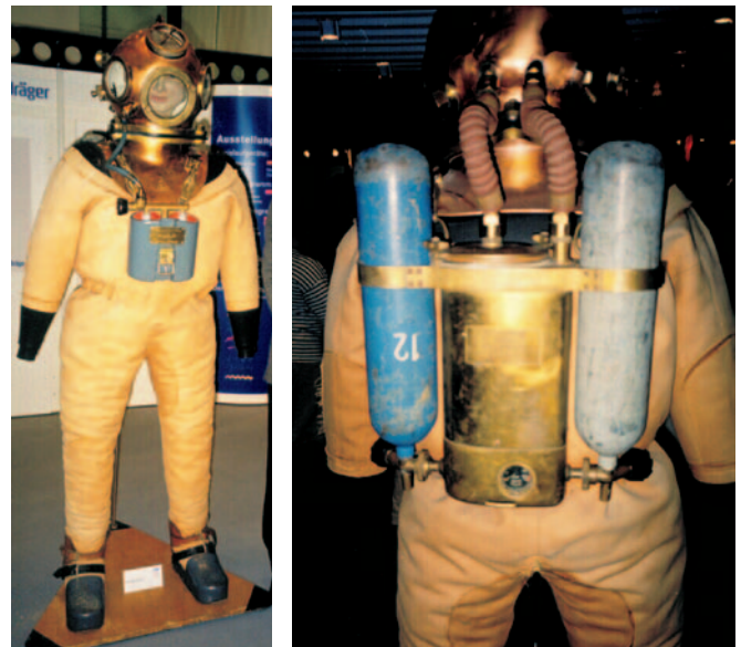
Photo 9. The diving apparatus DM 40 manufactured by Dräger 1915 (the own photography, courtesy Dräger AG Lübeck)
