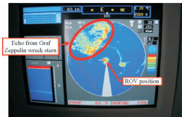
Fig. 3. ROV service desk in operation: sonar screen. Echo from the stern of the examined underwater object and vehicle position with respect to it are clearly visible (photo: S. Lipiński)
