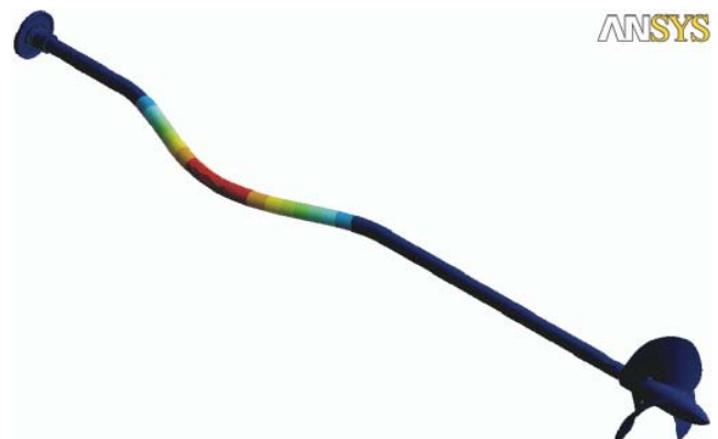
Fig. 1. Sample free vibration mode observed in the analysed propeller shaft
