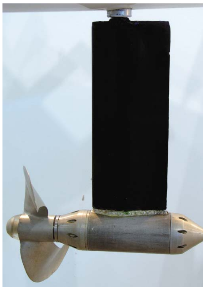
Fig. 14. The designed propeller in the arrangement with the pulling screw
