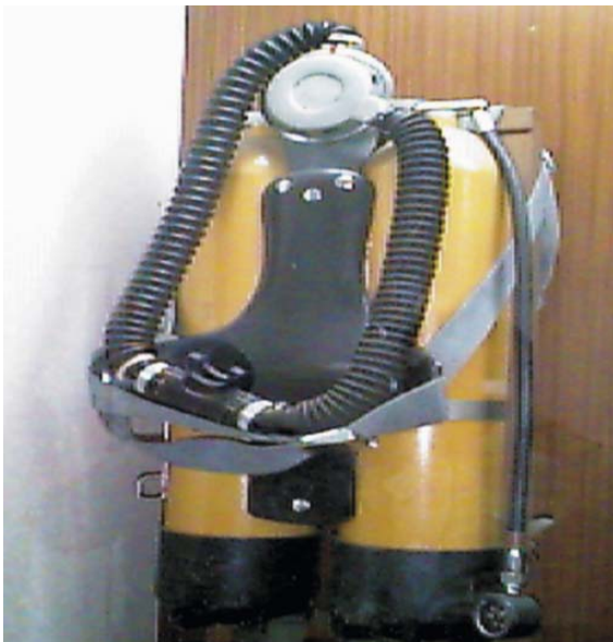
Photo 13. Diving apparatus PR-27 type SCUBA
