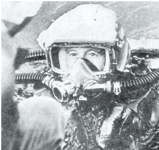
Photo 22. SCR applied in SealabIII [4]
