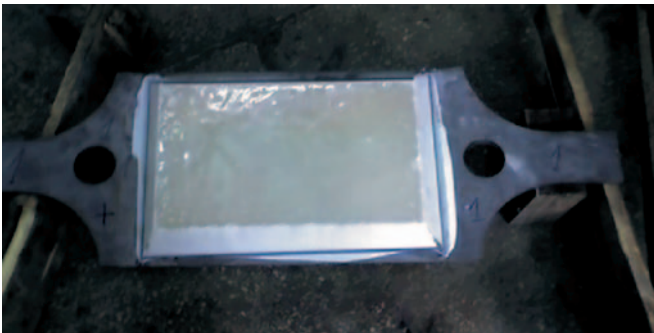
Fig. 8. Sample coated with polyurethane via RIM technique to be used for mechanical strength testing
