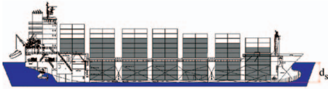
Fig. 7. Definition of the load line draught according to regulation 12A
