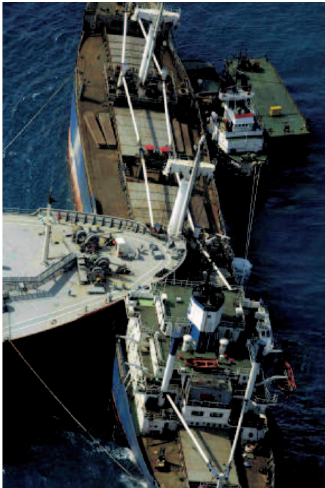
Fig. 2. A detail of side structure penetration during collision of m/t Gas Roman and m/v Springbok [2].
