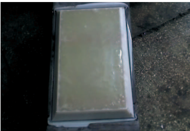
Fig. 10. Sample coated with polyurethane via RIM technique to be used for mechanical strength testing
