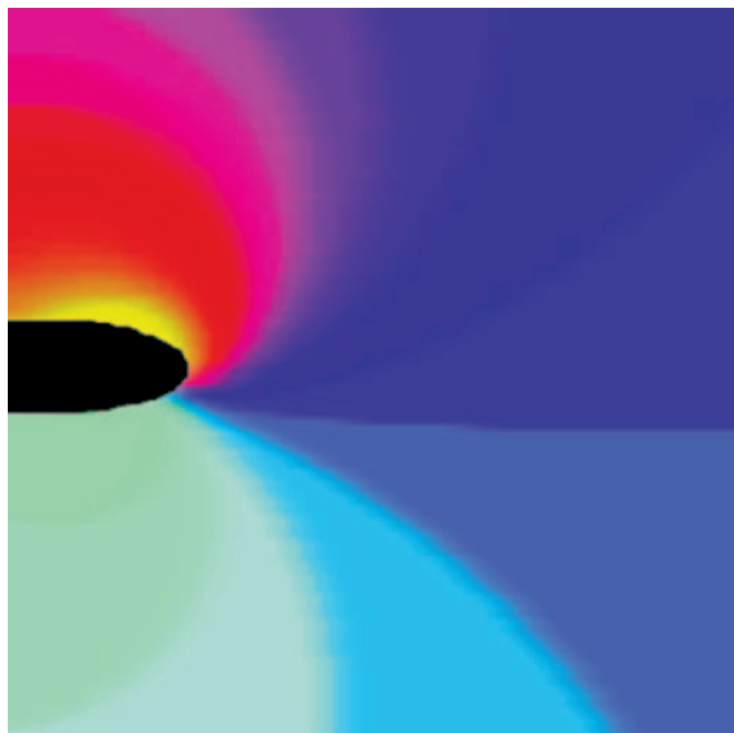
Fig. 6. Calculated pressure field around the rudder at zero deflection.
