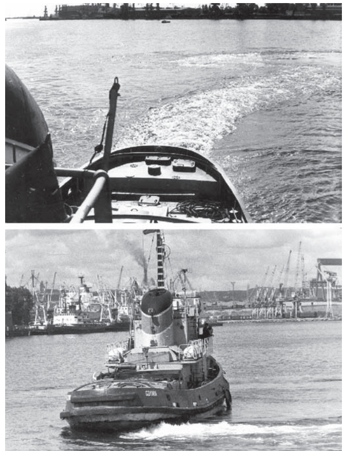
Fig. 4. Photo of Tug "Achilles" showing her manoeuvring ability and producing transverse force.
