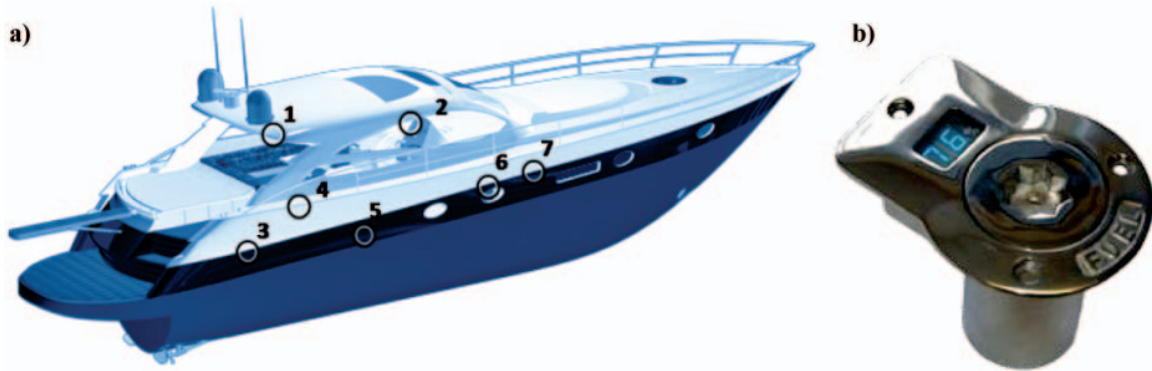
Fig. 5. a) 1 Lay-out of the most important elements of the Albatross Control and Management System on a 60 – feet motor yacht.
