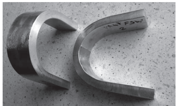
Fig. 2. A view of FSWmethod-welded specimens after bending tests
