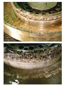
Fig. 8. Used silicone oil (solidified material) stuck to the casing of the viscous torsional vibration damper
