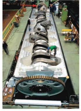
Fig. 2. a) 8S70MC-C diesel engine for ship propulsion [18],
