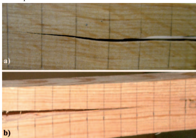
Rys. 11. Images of crack propagation surfaces in the specimens in the mode RL: a) natural wood, b) modified wood
