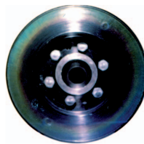
Photo 4. Image of an overheated and seized viscous torsional vibration damper, acc. tests made by the DAMPOL
