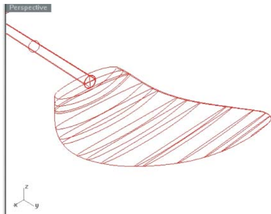
Fig. 3. Design of the model hydrofoil
