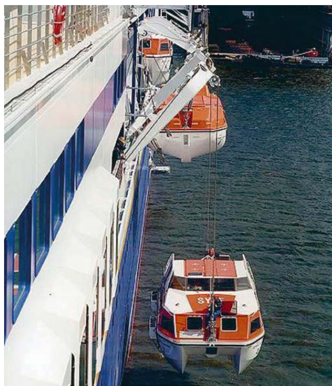
Fig. 1. View of the lifeboat and the luffing-jib davit during launching test
