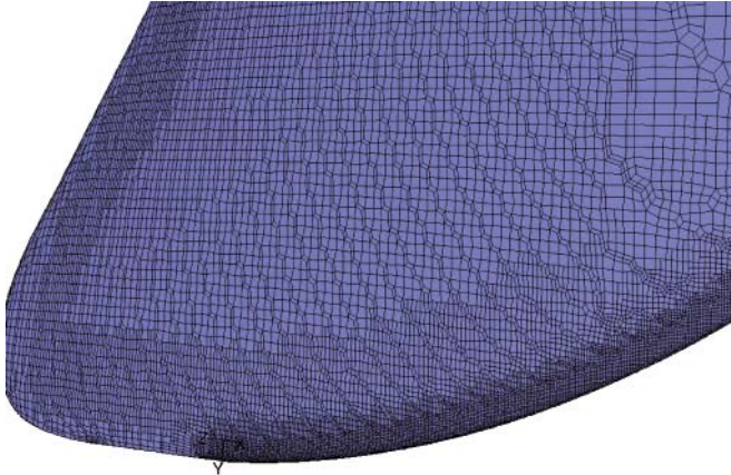
Fig. 2. Computational grid used in Fluent in the tip region of the hydrofoil
