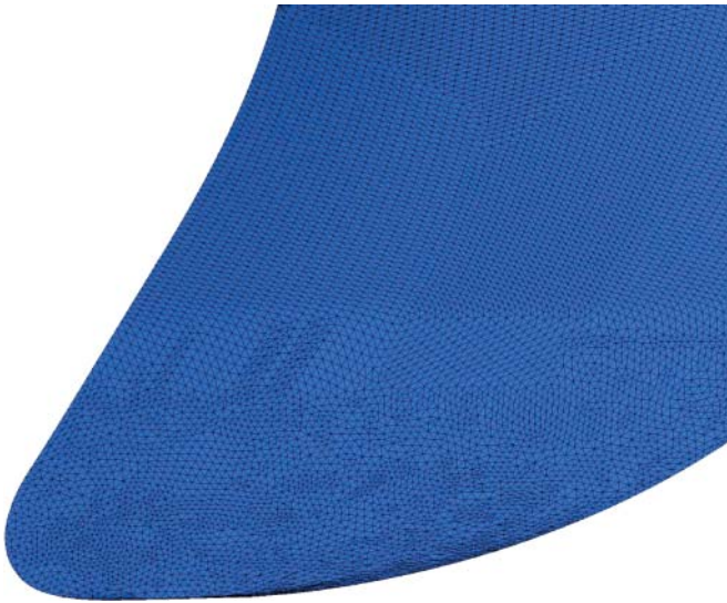
Fig. 4. Computational used in CFX in the tip region of the hydrofoil
