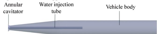
Fig. 1. Schematic geometry of vehicle model
