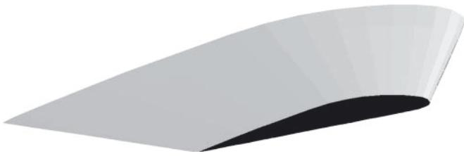
Fig. 5. Wing geometry modelled by the Autowing
