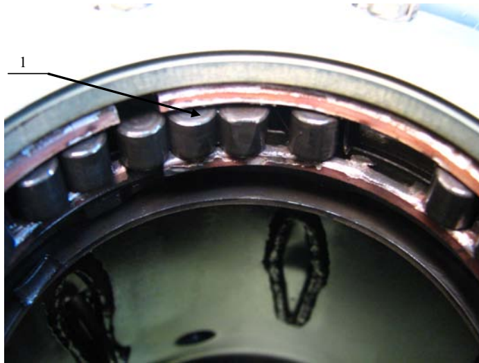
Fig. 7. The damaged central bearing diagnosed by means of FAM-C method: 1- interrupted ring of the spacer-separator
