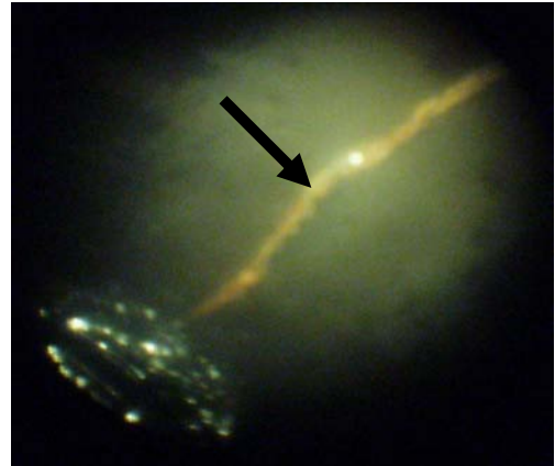
b) Cylinder liner sliding surface of four-stroke high-speed M503A ZVEZDA engine – cylinder liner cracks
