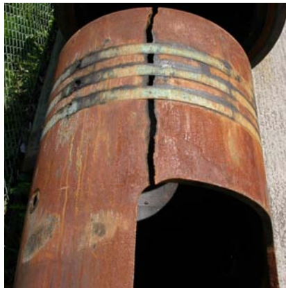
Fig 1. View of a cracked of piston skirt
