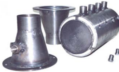
Fig. 6. Metallic enclosure of tested catalytic converter [3]
