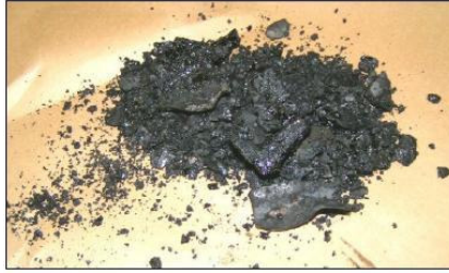
Fig. 3. Carbon deposits / asphalts taken from the exhaust gas outlet casing
