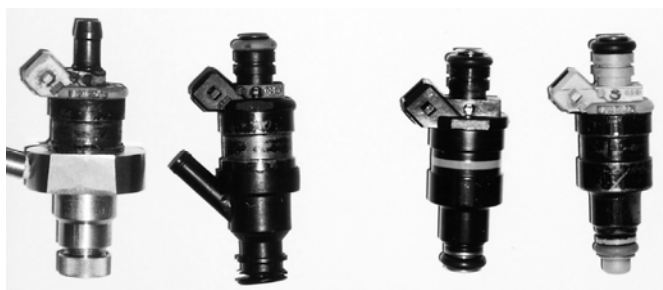
Fig. 4. Research injectors, on the left experimental injector with air assist
