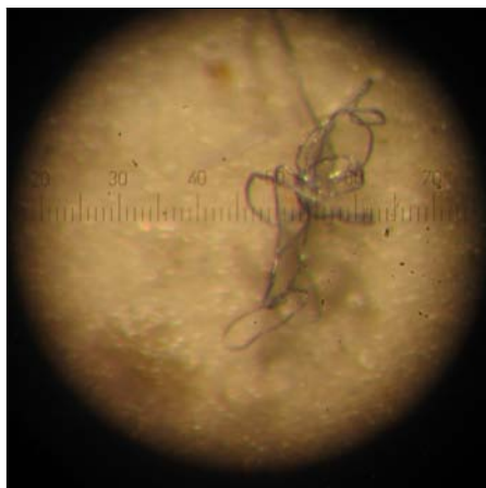
Fig. 4. The microscope view of the contaminant on the oil sample
