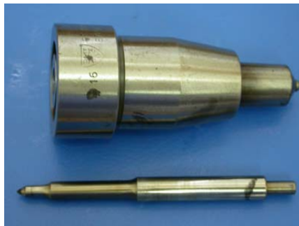
Fig. 2. Body and needle of injector nozzle tacked in investigations
