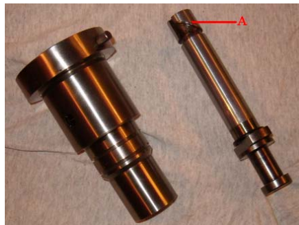
Fig. 5. Defect on the working edge of the precision pair of the plunger of the fuel pump (point A)
