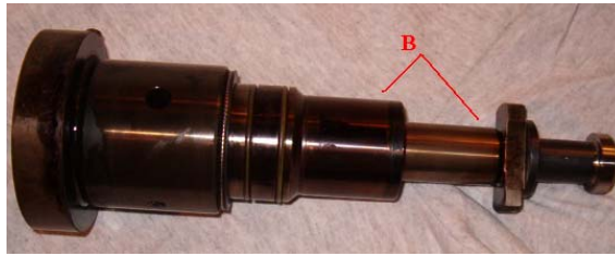
Fig 6 Discoloring of working surfaces of another precision pair due to too high temperature (surface B)
