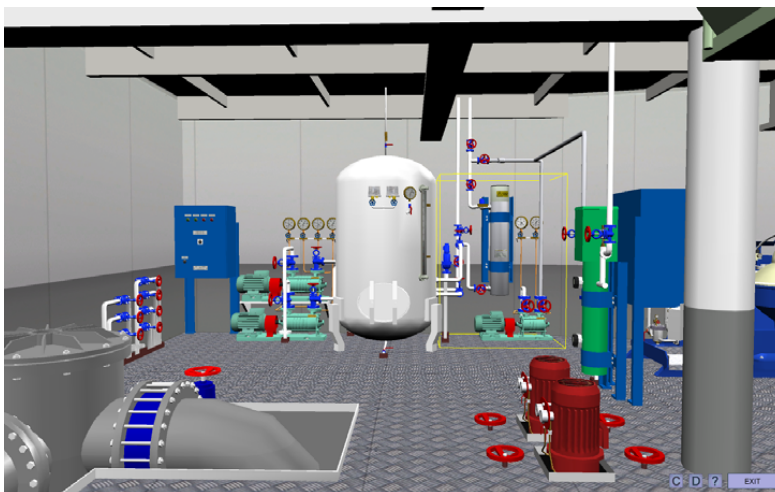
Fig. 6 MED3DH Engine Room Simulator - Hydrophore installation
