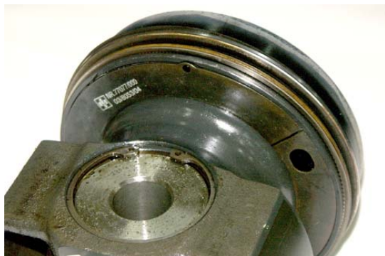
Fig. 1. The piston of the Caterpillar 3516A engine: a) the view of the piston ; b) the scheme of ring mount in the
