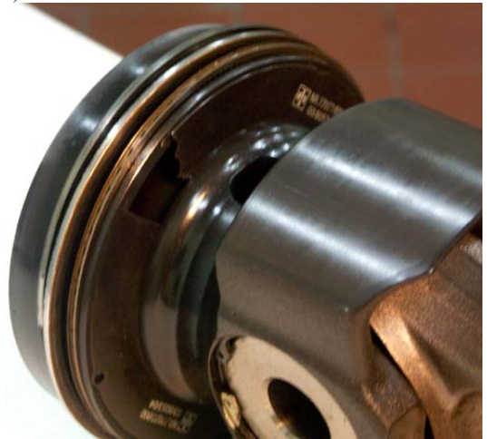
Fig. 5. A view of the piston after failure on the 8 th cylinder
