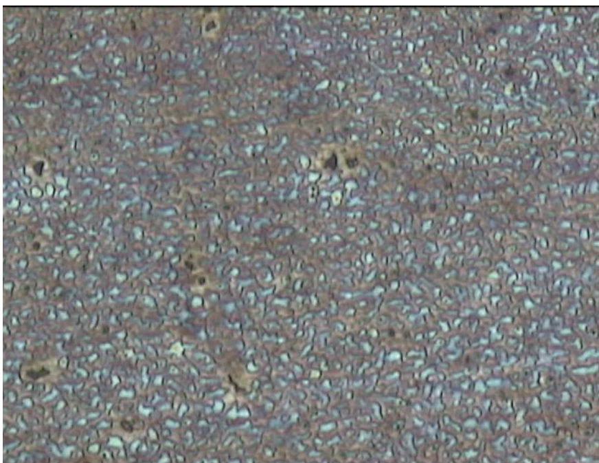
Fig. 6 Microstructure of thrust ring material in quenched and tempered state: bainitic-sorbite structure; etched with nital, magnification 500x
