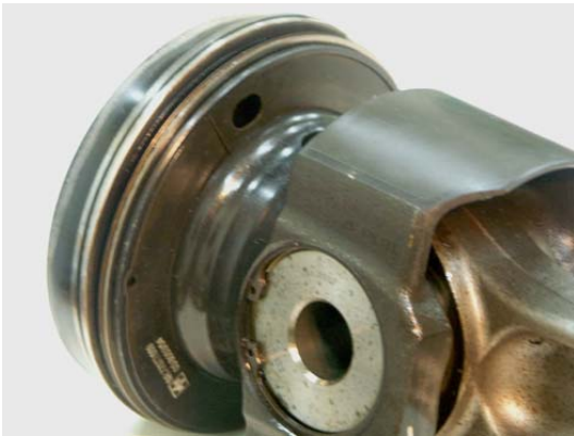
Fig. 5. A view of the piston after failure on the 8 th cylinder
