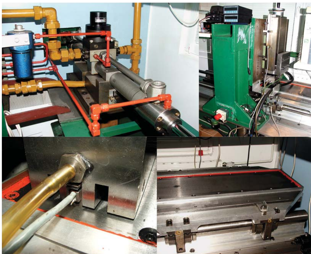
Fig. 11. View of the test stand, upper left corner – hydraulic drive, upper right corner – saddle with piston model attached, lower left corner – piston model with attached slat, lower right corner – the plate that simulates the cylinder liner surface
