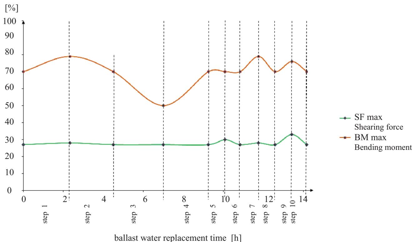
Drž. 6. Diagram of maximum values of the shearing forces and bending moments in the ship hull initial during the ballast water replacements – the m/v „Orla” ship
