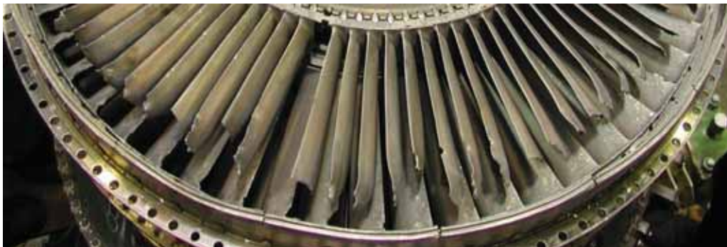
Fig. 2. Example forms of temperature defects demonstrated by vanes of the turbine rotor [6]
