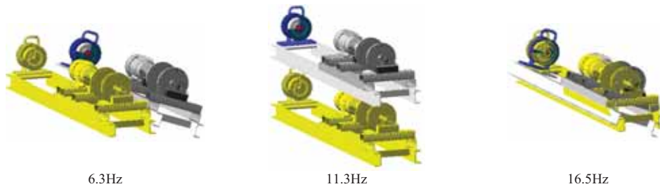
Fig. 2.4. The forms of norma mode vibrations – equilibrium position marked yellow
