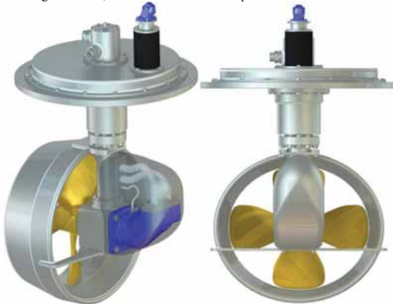
Fig. 5. Axonometric (with transparent fairwater cap) and central projection view of the azimuth thruster.
