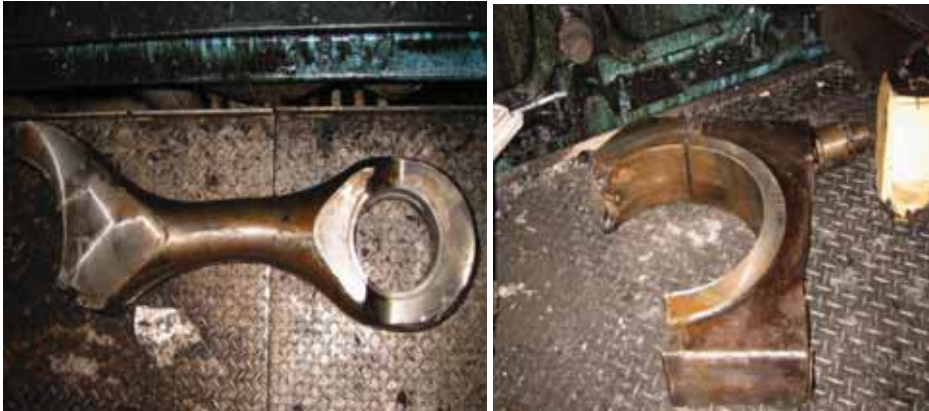
Fig 6. The photographs show the severed connecting-rod bases of the Bergen- Diesel engines on one of the “Seismic Research” type ships.
