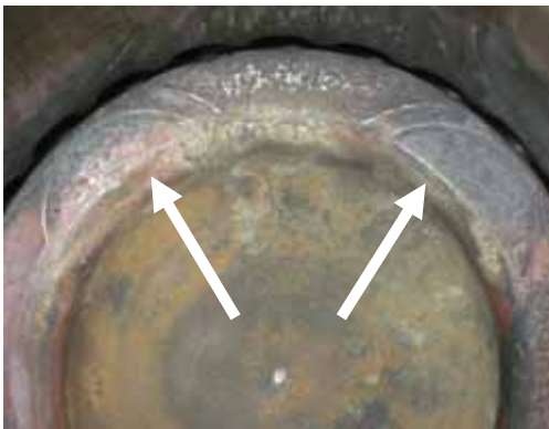
c) piston head – traces of the piston strokes over the valves (a state after the “water hammer”)
