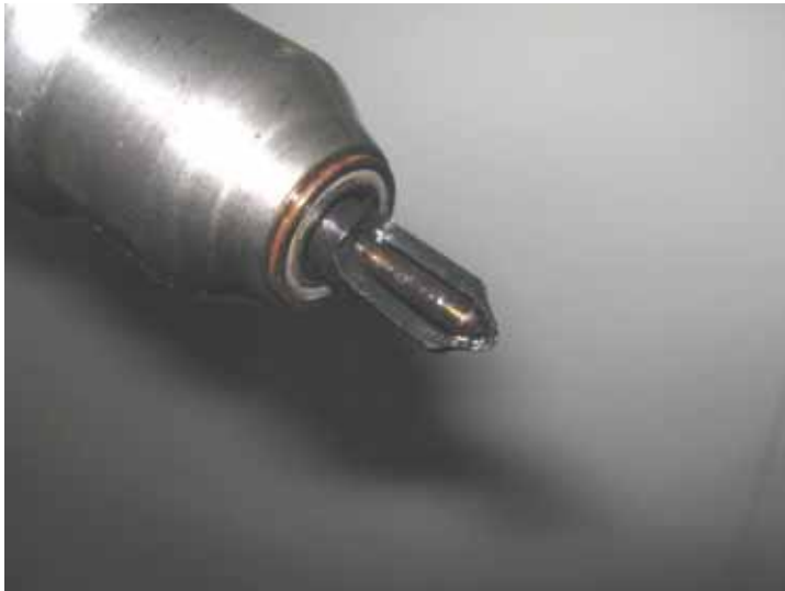
Fig. 4. A view of the damaged atomizer in a injector pump of the Caterpillar engine
