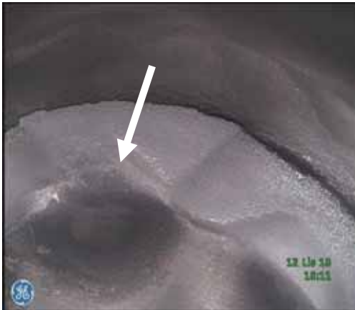
a) piston head – traces of the fuel after-burning
