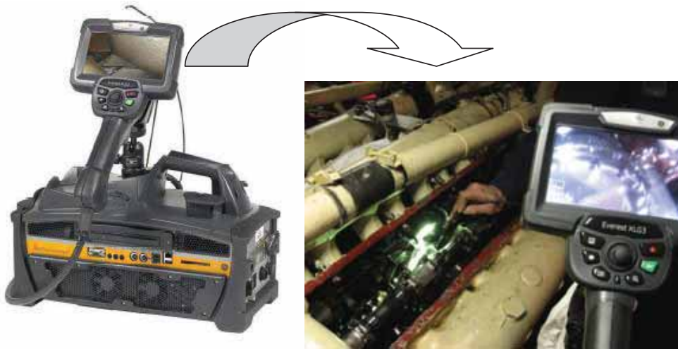
Fig. 1. Engine's examination by means of EVEREST XLG3 digital measuring videoendoscope [12]
