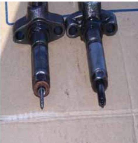
Fig. 2. An example of damage (breakaway) of a part of the atomizer body caused by the improper quality of fuel
