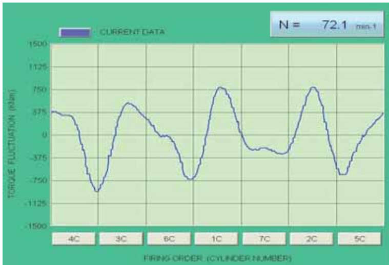
Fig. 9. Course of torque fluctuation t in particular cylinders at 72 rev/min and load index 80% for large marine diesel engine Mitsubishi UEC 7L85II
