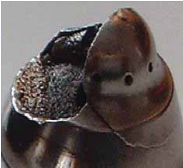
Fig. 1. Partial (fig. a) and total (fig. b) breakaway of the atomizer nipple
