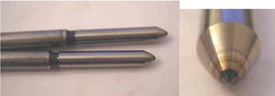
Figure 9 Scorched atomizer needle cones.
