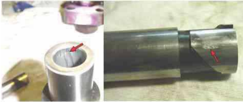
Fig. 11. Seizing of a precision pair of a (new) injection pump after four hours of operation due to very low quality of manufacturing of parts (Chinese manufacturer)
