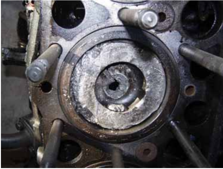
Fig. 3. Damage of the piston and engine body being the result of the breakaway of the lower part of the atomizer body (from Fig. 2)
