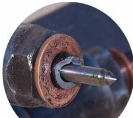
Fig. 2. An example of damage (breakaway) of a part of the atomizer body caused by the improper quality of fuel
