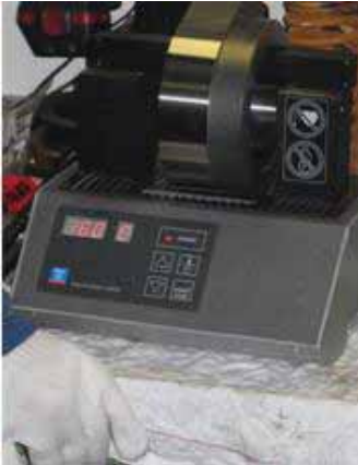
Fig. 3. Warming up of the shaft gear cam with the use of an induction heater
