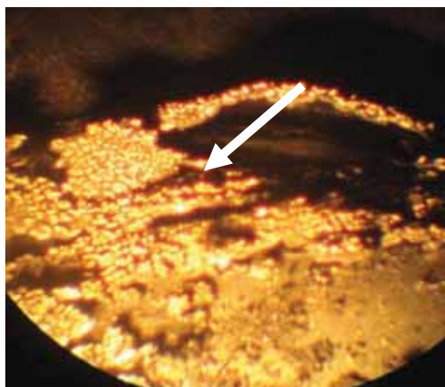
e) piston head – a thick layer of the carbon deposit
