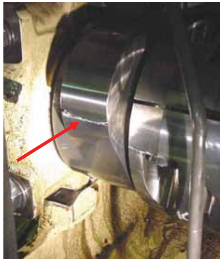
Fig. 2. The crack on the cam of the fuel pump (marked with an arrow)
