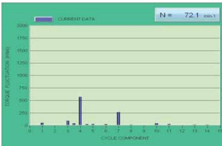
Fig. 10. FFT of torque fluctuation t in particular cylinders at 72 rev/min and load index 80% for large marine diesel engine Mitsubishi UEC 7L85II
