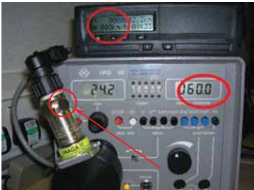
Fig. 4. The location of the magnet used to manipulate the indications of digital recording equipment
