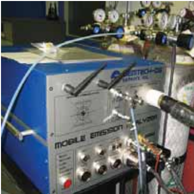
Fig. 4. View of the exhaust emission analyzer
