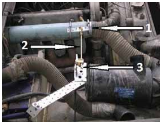
Fig. 5. Fixing the measuring system in the engine compartment, 1 – arm mounting location, 2 – the potentiometer arm connecting, 3 – potentiometer
