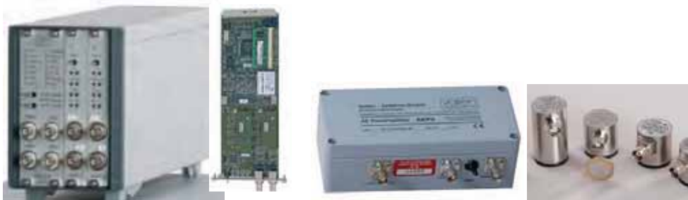
Fig. 6. The AE method measurement set by enterprise Vallen
