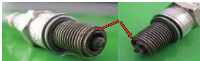
Fig. 9. Failure of removing the spark plug side electrode
