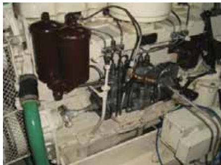
Fig.4. Engine SW400 type fuel system with three-way pass valve to cut off fuel supply to the chosen injector
