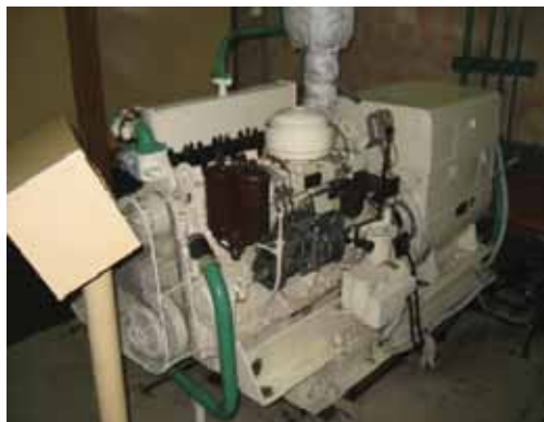
Fig. 1. General view of marine generating set ZE400/52 mounted on the test bed
