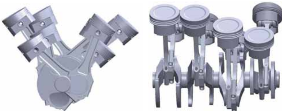
Fig. 3. 3D model of a piston-crank system in a V-VR8 engine
