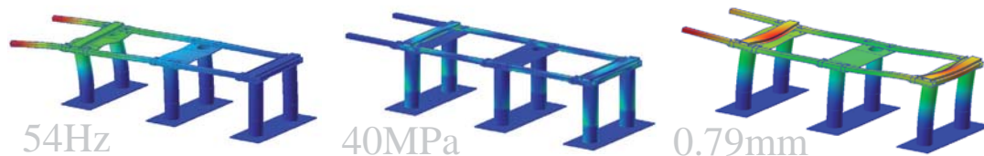
Fig. 6. The lowest expected frequency of the screen support structure's own, natural vibrations following its upgrade and the stresses and strains in cross-sections
