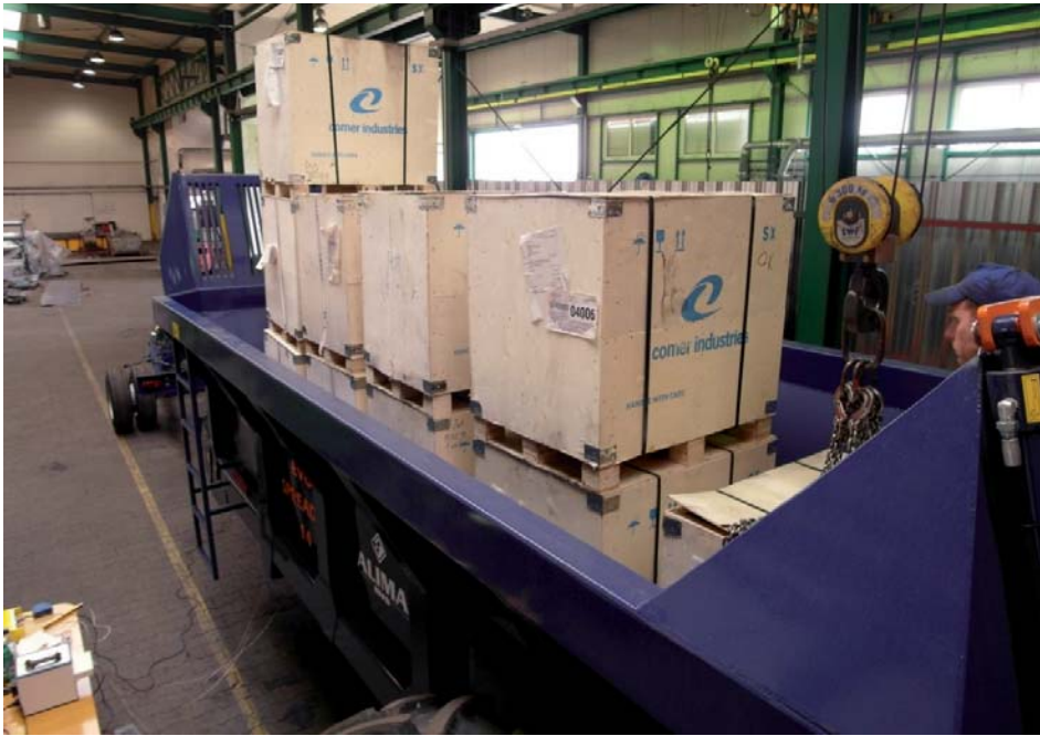
Fig. 6. Manner of loading of the tested frame structure
