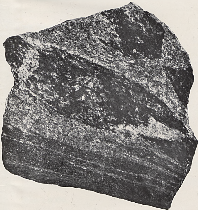
Fig. 2. Brecciated and banded boundary form of gabbro. — Nat. size. — North slope of the Gellivare Dundret.
