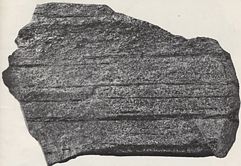
Fig. 1. Gneissoid syenite, with stripes of magnetite. — \frac{1}{2} nat. size. — Linné adit.
