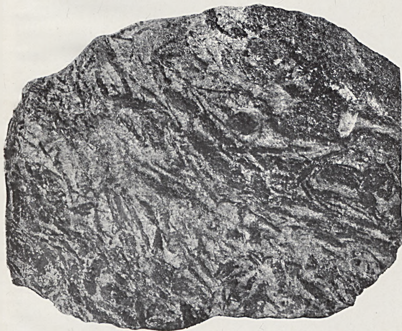
Fig. 2. »Skarn» rock, with granular felspar and radiating amphibole crystals. — \frac{1}{3} nat. size. — Fredrika mine, Kapten ore.
