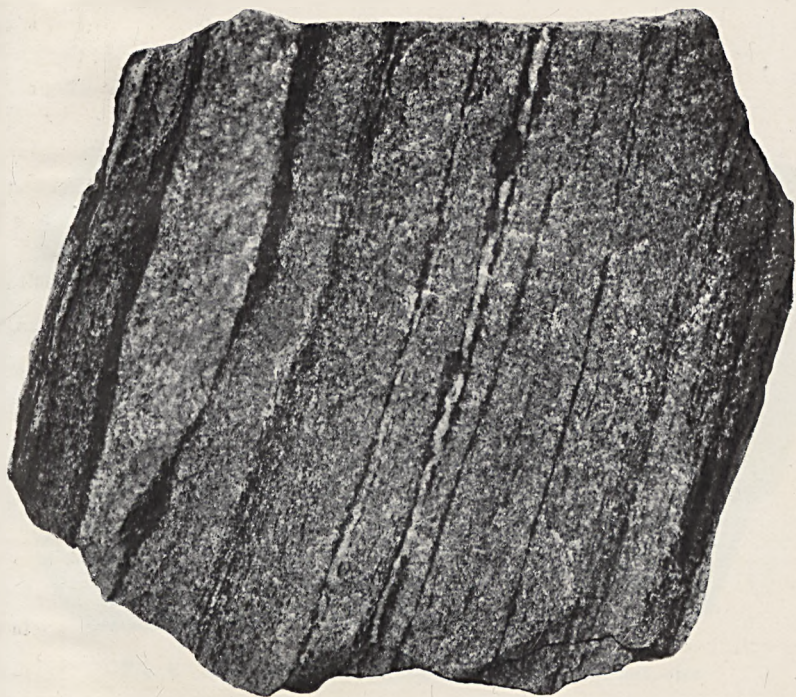
Fig. 2. Gneissoid syenite rock, with stripes of hornblende and segregations of felspar. — Length section, natural size. — Foot wall of the Baron mine.
