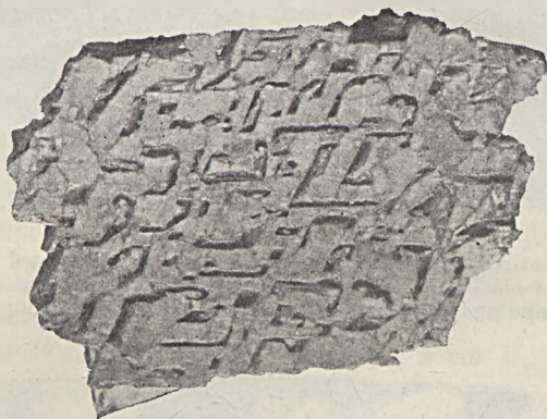
Fig. 22. Felspar with graphic texture and the quartzes removed. Section parallel (010). The vertical axis of the felspar stands in the fig. upright. (After A. G. HÖGBOM.)
