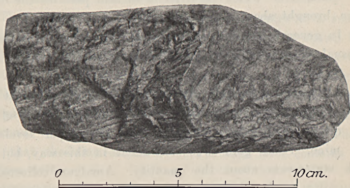
Fig. 2. Brecciated structure of the zinc deposits in dolomite.
