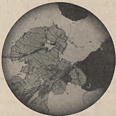
Fig. 2. Gahnite, enclosed in quartz. The dark mineral is sphalerite. One nicol. Magn. 24 diam.
