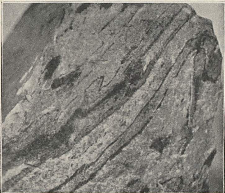
Fig. 2. Skarn-banded soda granulite from Tilas' adit, Högberget, Persberg. Nat. size.
