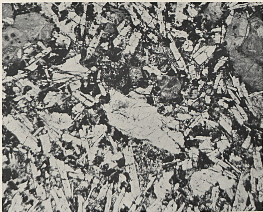
Fig. 2. Corroded labradorite phenocrysts in kenningite. Serpentinized olivine crystals appear gray. Ord. light. Magnif. \times 40 .
