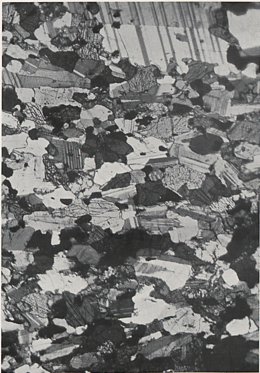
Marginal part of porphyritic noritic gabbro-dike. A labradorite phenocryst occupies the top part of the picture. Nic. +. Magnif. \times 40 .
