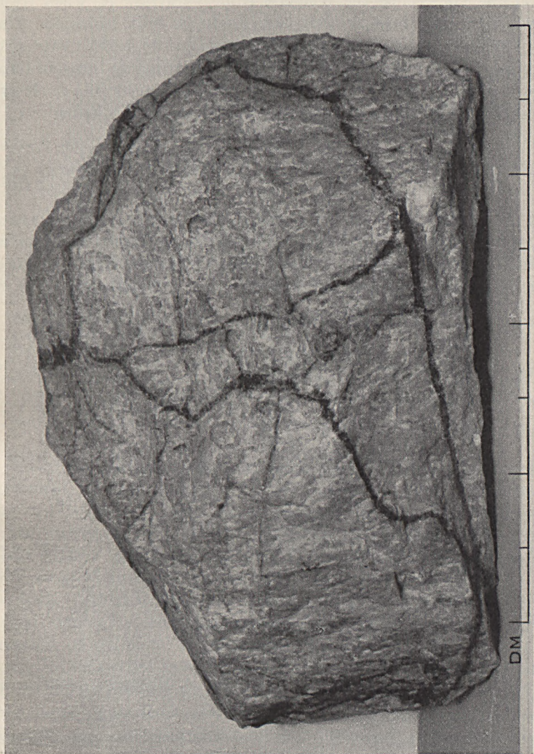
Fig. 1. Specimen of pollucite, Varuträsk, intersected by dark veins of albite. Weight of block 75 kg. (About \frac{1}{4} , nat. size.)
