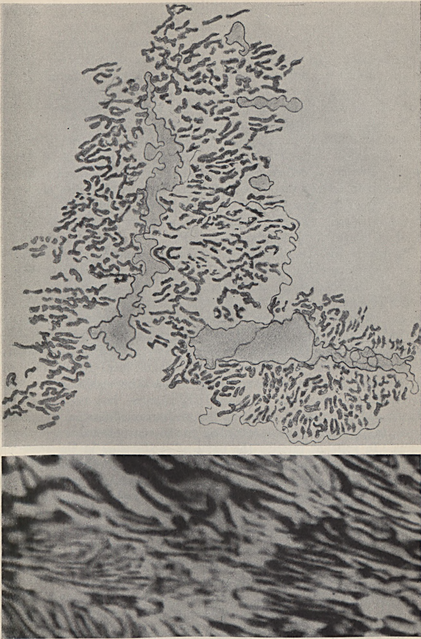
Fig. 6. Upper fig. microscopic drawing by MARGIT ROSENBERG of albite-eucryptite symplektite from caesium diaspodumene vein in pollucite Varutrask. ( 200 \times 1 .) Dark fibres eucryptite, white albite, shadowed parts quartz. Lower fig. microscopic photo of Branchville albite-eucryptite symplektite, enlarged to same scale.
