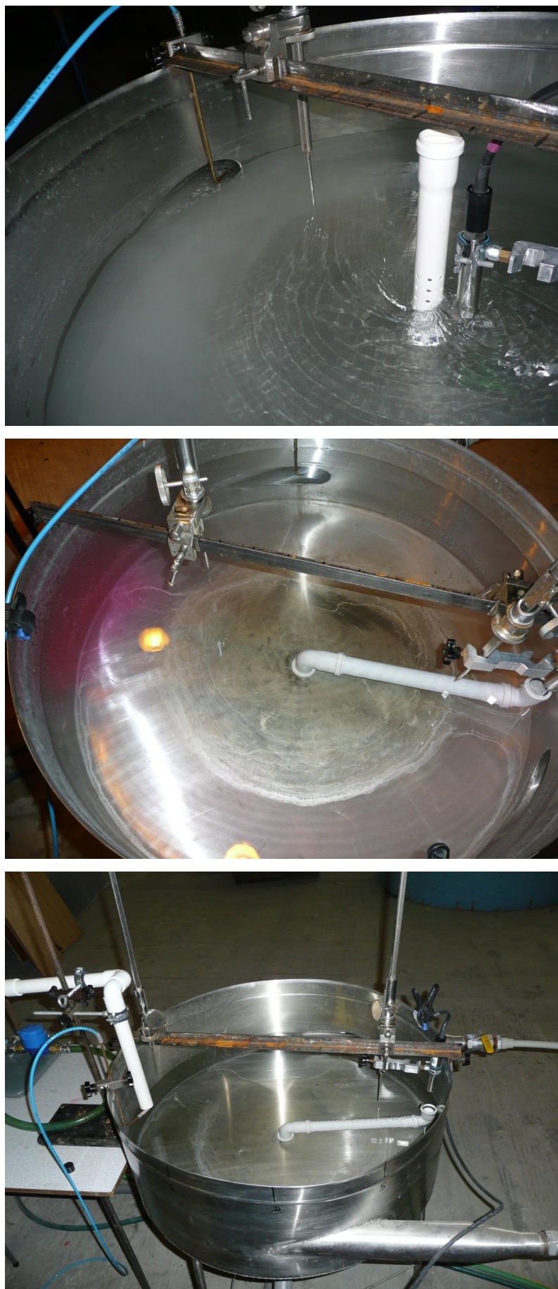
Fig. 9.3. Inlet-outlet combinations used in tracer measurements (“P” series, “T” series, “W” series)
