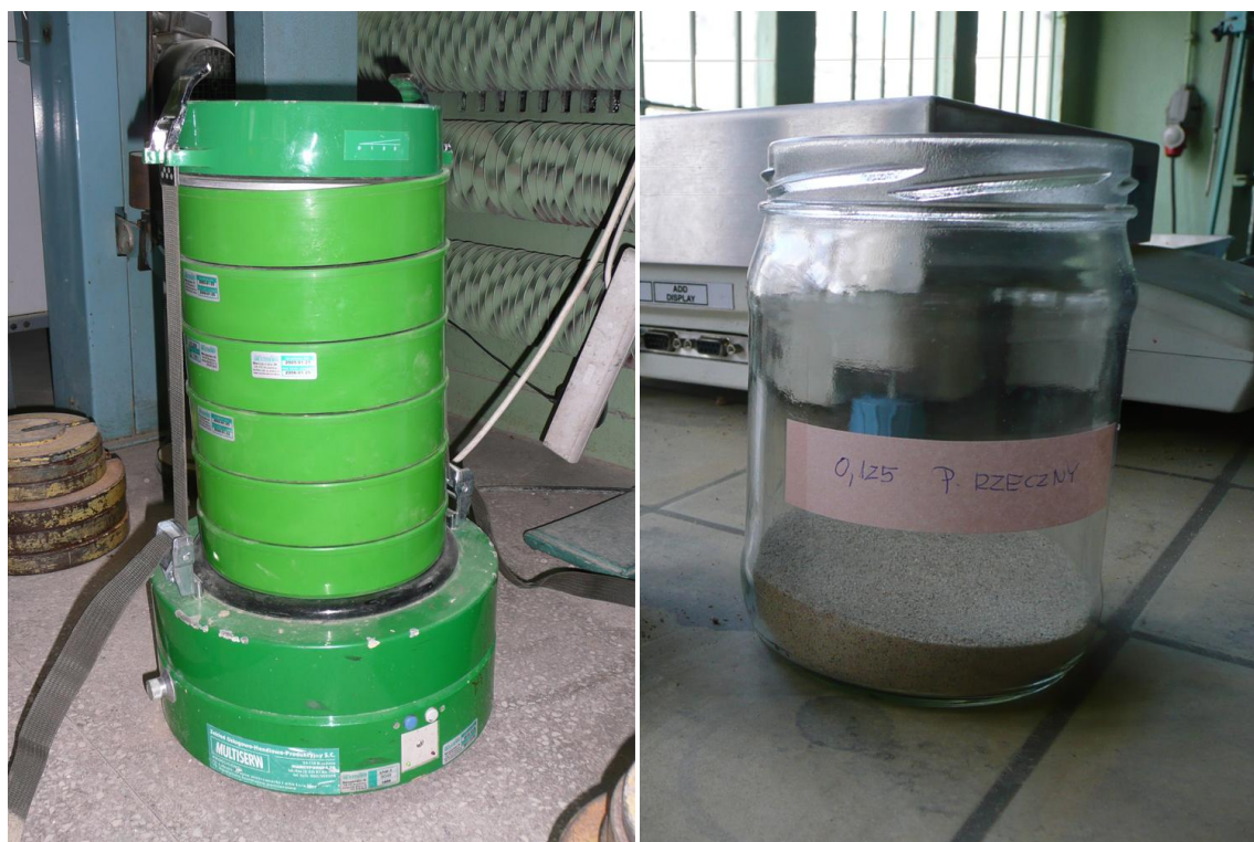
Fig. 10.3. Preparation of sand material for efficiency tests (sieve analysis, single sand portion)
