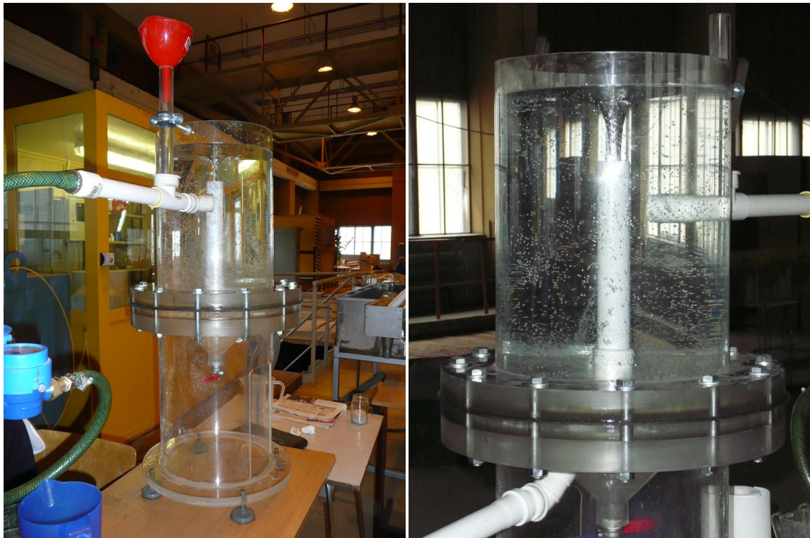
Fig. 10.1. Laboratory prototype of vortex separator
