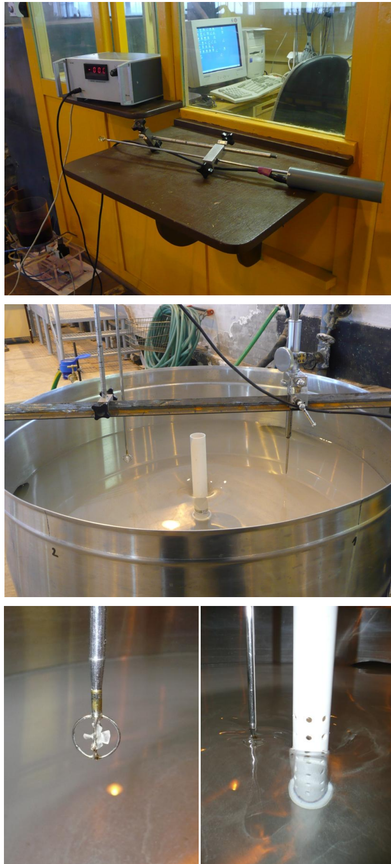
Fig. 5.6. Equipment for velocity measurements (computer station, micro propeller current meter, water level gauge, perforated outlet pipe)
