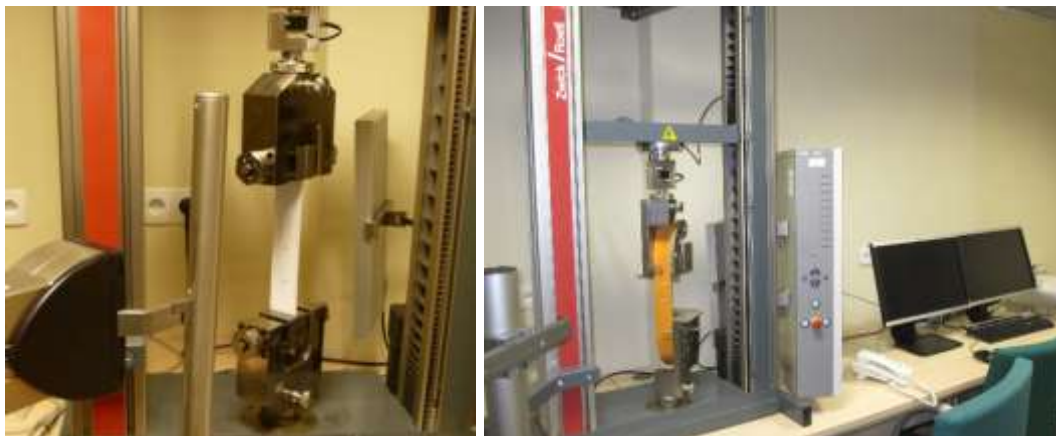
Fig. 5.1. Zwick Z020 with video-extensometer
