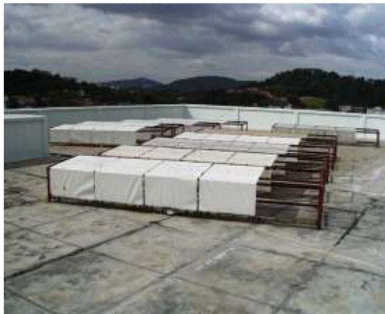
Fig. 3.3. Example of natural weathering- test racks with fabrics at exposure location on the fifth story of a building in Malaysia [196]
