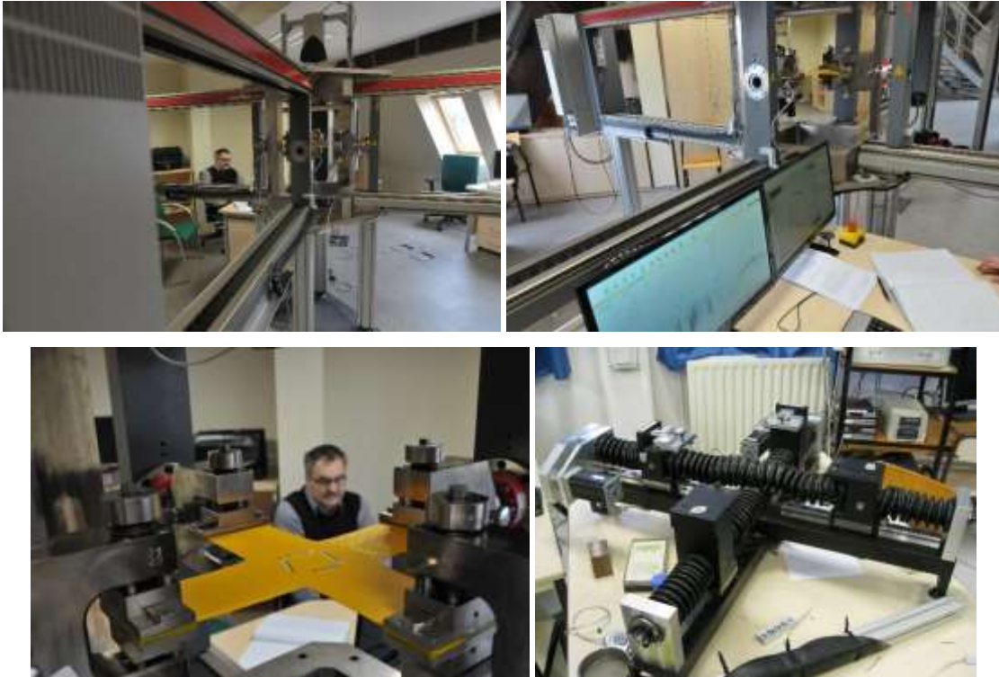
Fig. 5.2. Zwick strength machines for biaxial tests with video-extensometer
