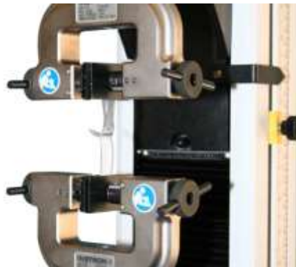
Fig. 2.9. Seam test of two fabric pieces welded together ([108])
