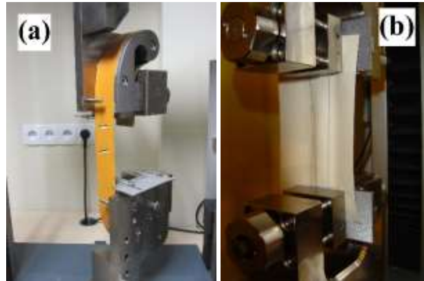
Fig. 2.3. Uniaxial tensile tests of technical fabrics (Gdansk University of Technology): (a) cut strip method; (b) grab test method
