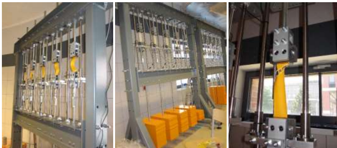
Fig. 5.4. Experimental 10-stands machine for creep tests
