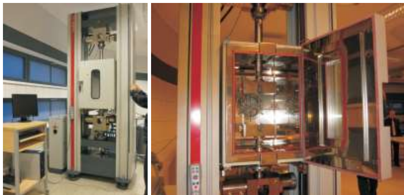
Fig. 5.3. Zwick Z400 with thermal chamber
