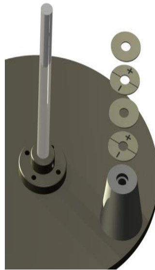
Fig. 2.25 Hybrid piezoelectric motor - orientation of the ceramics and the electrode
