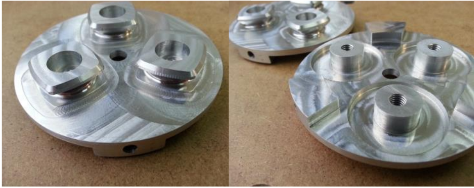
Fig. 7.1 The new counter-mass manufactured on the milling machine (CNC)
