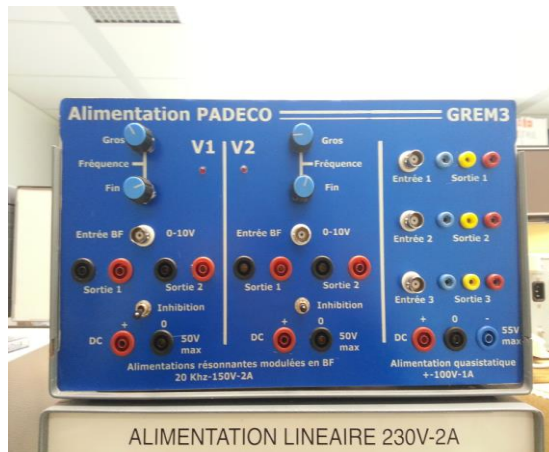
Fig. 6.29 Linear amplifier power supply for piezoelectric motors - developed in LAPLACE Laboratory (INP-ENSEEIH, Toulouse)
