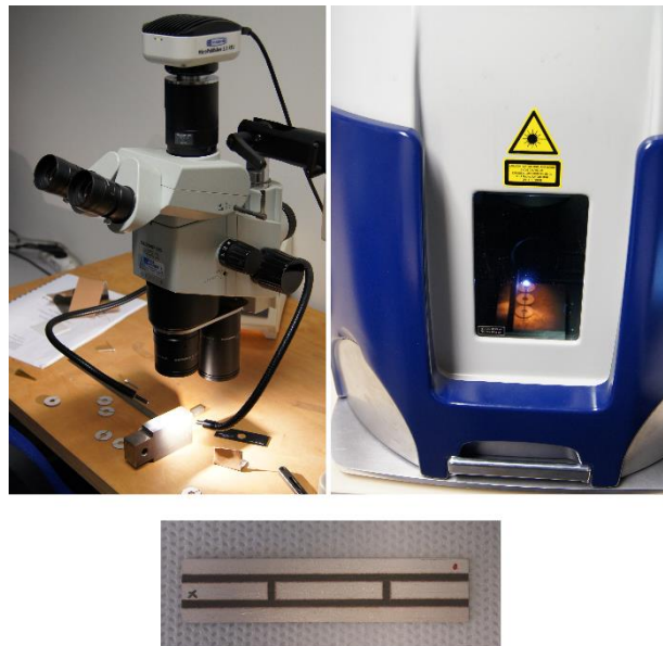
Figure 3.13 Sectorization process: upper right – laser cutting system; upper left – inspection of the depth of the cut; lower – sectorized ceramic
