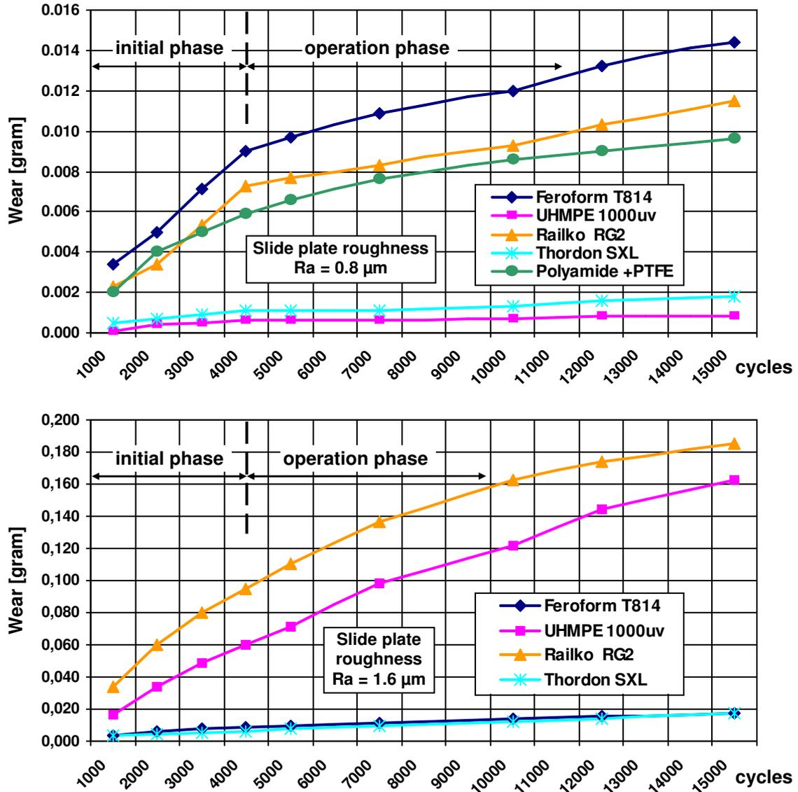
Fig. 87. Cumulative wear of synthetic materials on slide plates of different initial roughness
