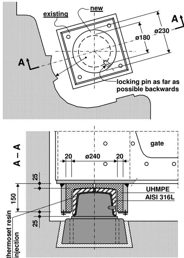
**Fig. 102.** New bottom pivot of Lock III in the Wilhelmina Canal in Tilburg
