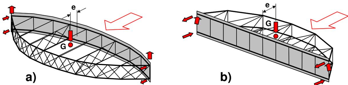
**Fig. 5.** Gate support systems in regard of vertical loads of the:
