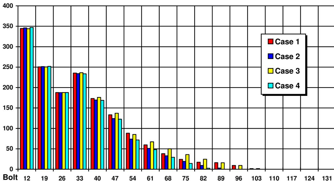
**Fig. 74.** Bolt tension (kN) distribution in four contact cases for the model from Fig. 72 (b)
