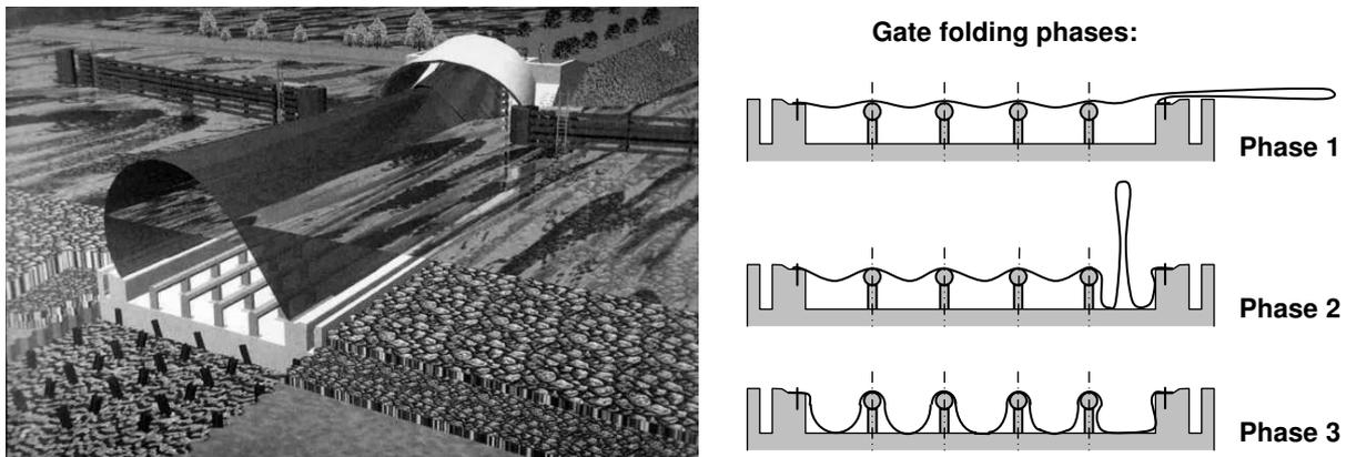
**Fig. 75.** Ramspol Dam: gate closed position (left) and phases of gate folding (right)
