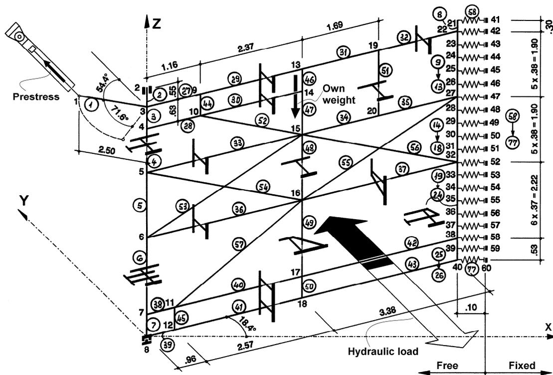
**Fig. 64.** Structural analysis model for the mitre gates of Naviduct Enkhuizen
