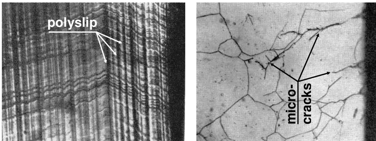
**Fig. 94.** Aluminum-copper (left) and stainless steel (right) crystalline structure shaped by fatigue, respectively  $\sim 800$  and  $\sim 200$  x enlarged, [103]
