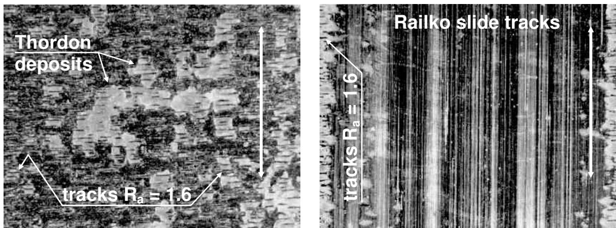
Fig. 88. Tracks on stainless steel slide plates: left Thordon, right Railko (10 x enlarged), [49]
