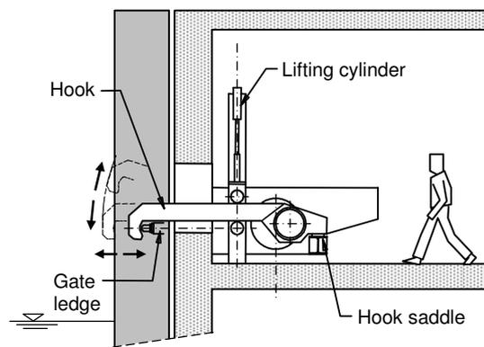
**Fig. 19.** Gate locking in the Yacht Lock in the Kramer
