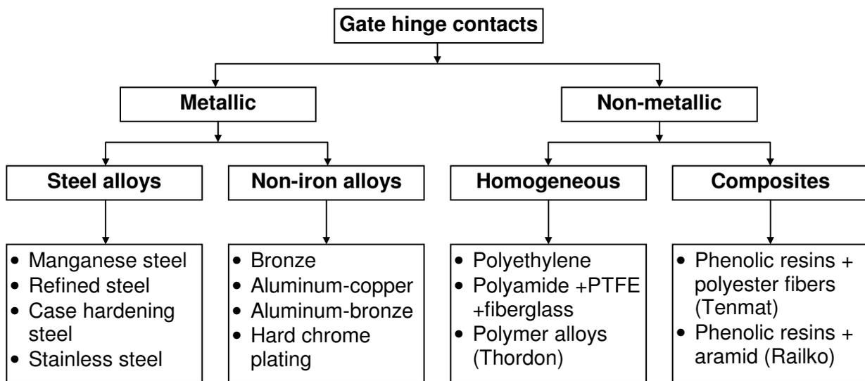
**Fig. 100.** Simple classification of the investigated contact materials
