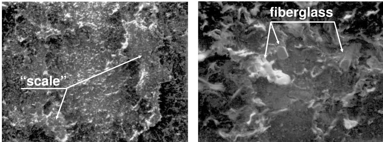
**Fig. 99.** Polyamide structure from a gate worn bearing, left ~50 x and right ~400 x enlarged, [89]
