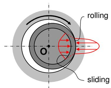
**Fig. 55.** Shaft in a bushing
