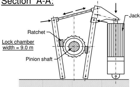
**Fig. 23.** Gate locking in the Schied Canal Lock in Schiedam
