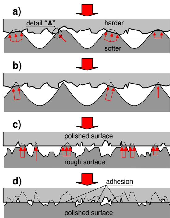
**Fig. 57.** Contacts on segment level, examples (enlarged:  $l/h \approx 10/500x$ )
