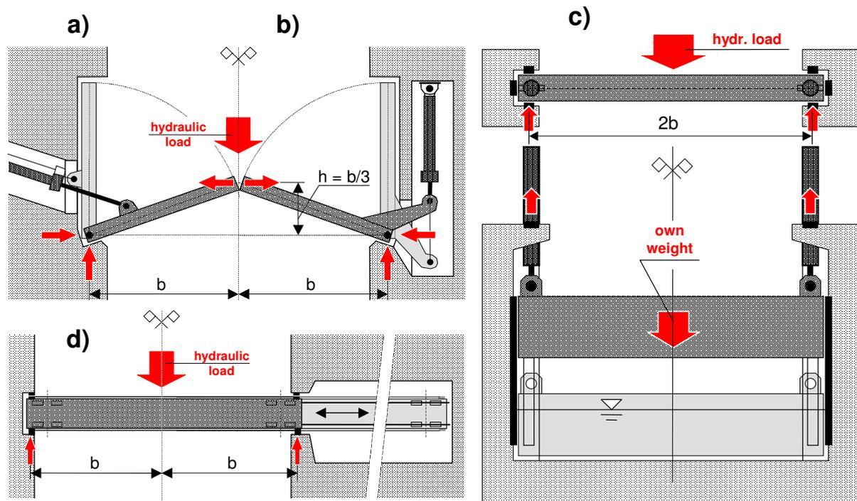
**Fig. 3.** Gate types for a barrier on the Meuse-Waal Canal; and for a navigation lock on the Meuse:
