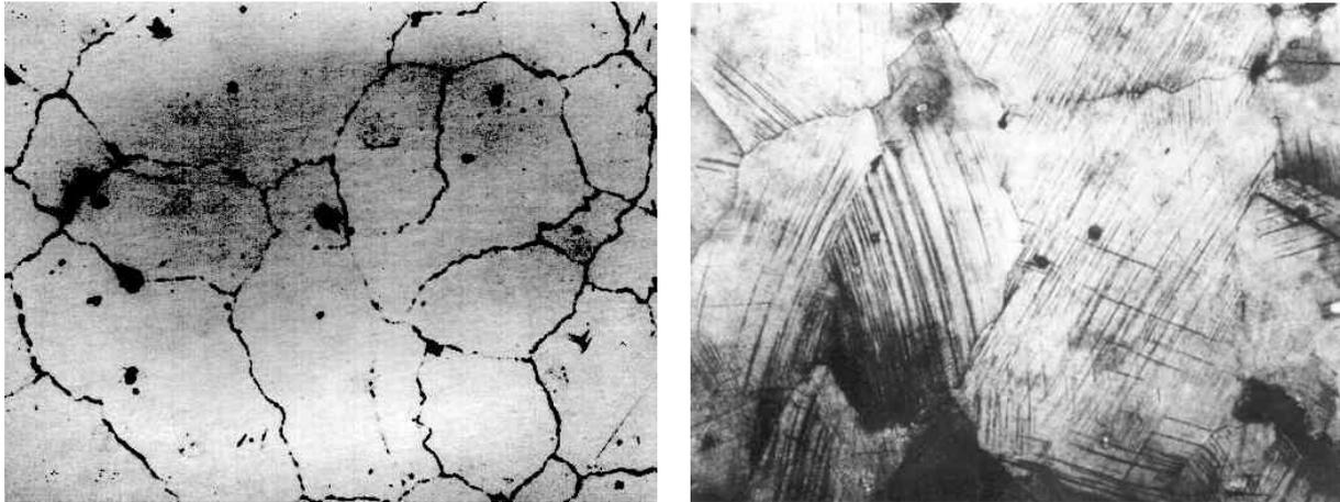
**Fig. 93.** Manganese steel crystalline structure far from (left) and on (right) the deformed surface, respectively  $\sim 80$  and  $\sim 160$  x enlarged, [49]
