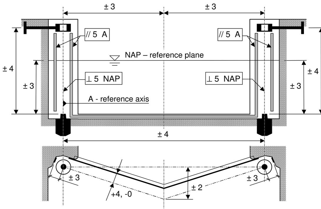
Fig. 9. Dimensional tolerances for a mitre gate contact items in a chamber – example
