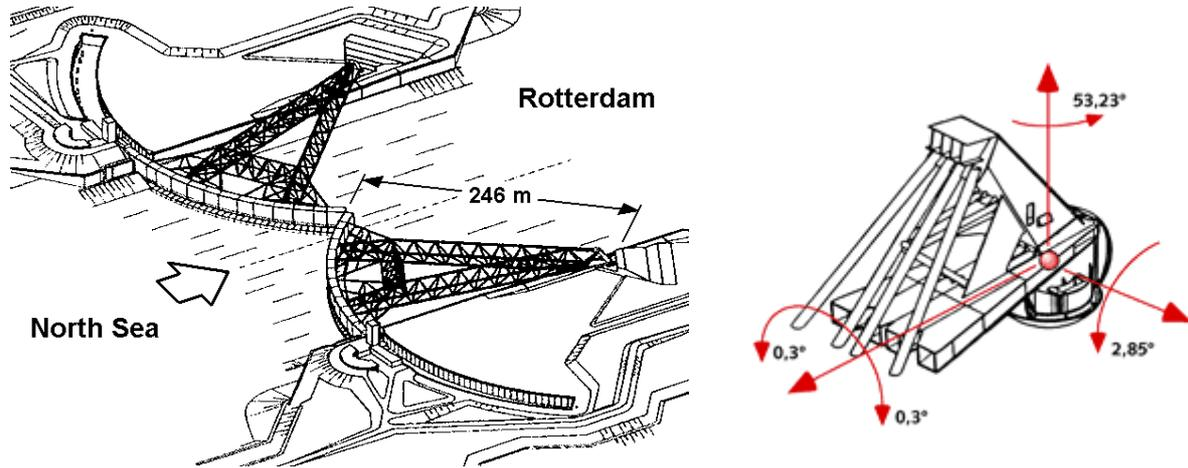
**Fig. 69.** The New Waterway Barrier and the support hinge of its sector gate
