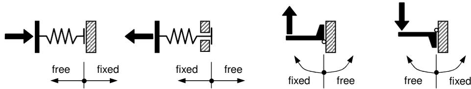
**Fig. 65.** Two examples of conditional DOF fixities
