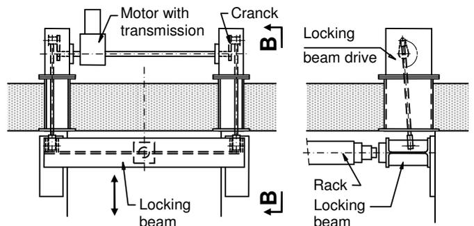
**Fig. 24.** Gate locking in the Merchants' Lock in Den Helder
