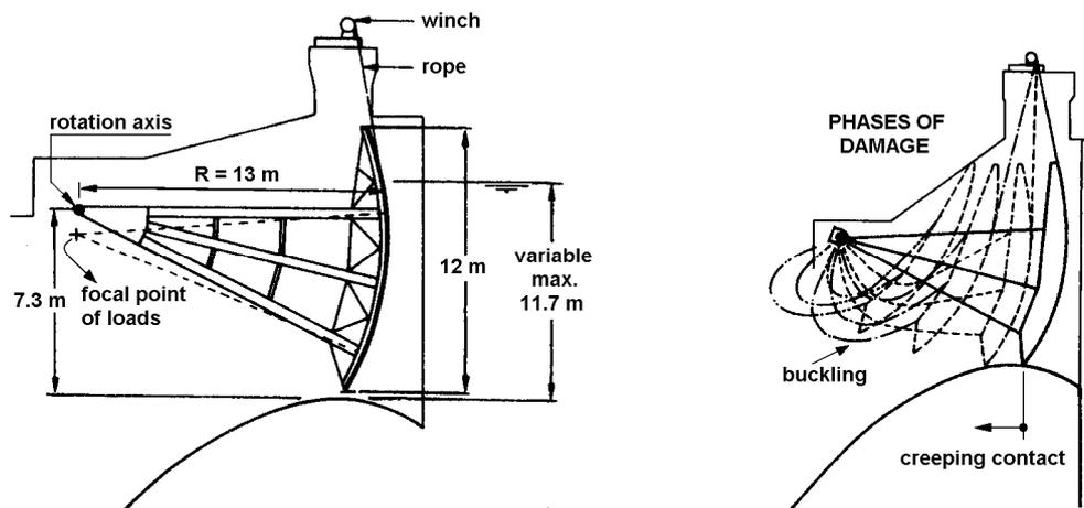
**Fig. 51.** Contact creep and damage of the Wachi-Dam tainter gate in Japan.
