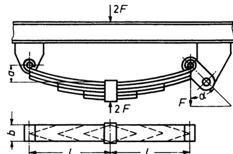
**Fig. 113.** Spring support of a railway wagon
