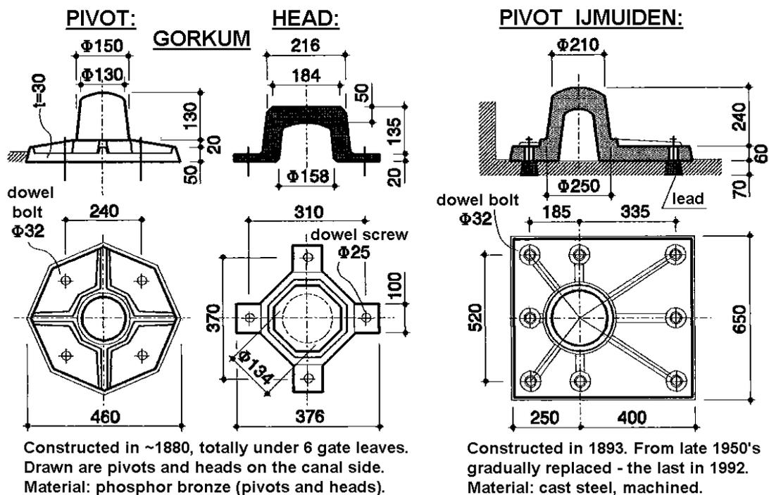
**Fig. 79.** Typical mitre gate bottom pivots from the end of 19<sup>th</sup> century in the Netherlands
