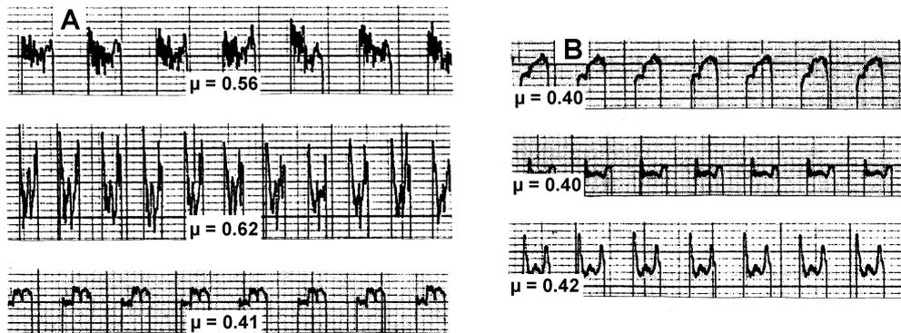
**Fig. 91.** Variation of friction force in single load cycles during testing
