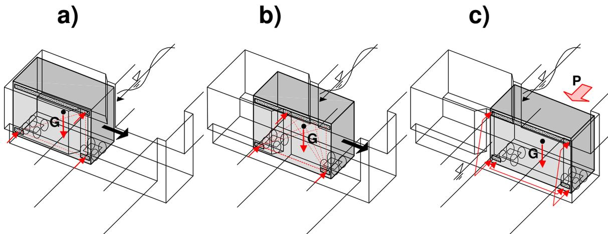
**Fig. 16.** Systems and supporting conditions of a rolling gate during closing
