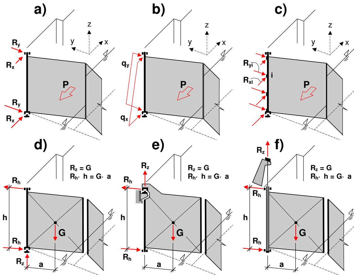
**Fig. 4.** Gate support systems in regard of hydraulic load (above) and own weight (below)
