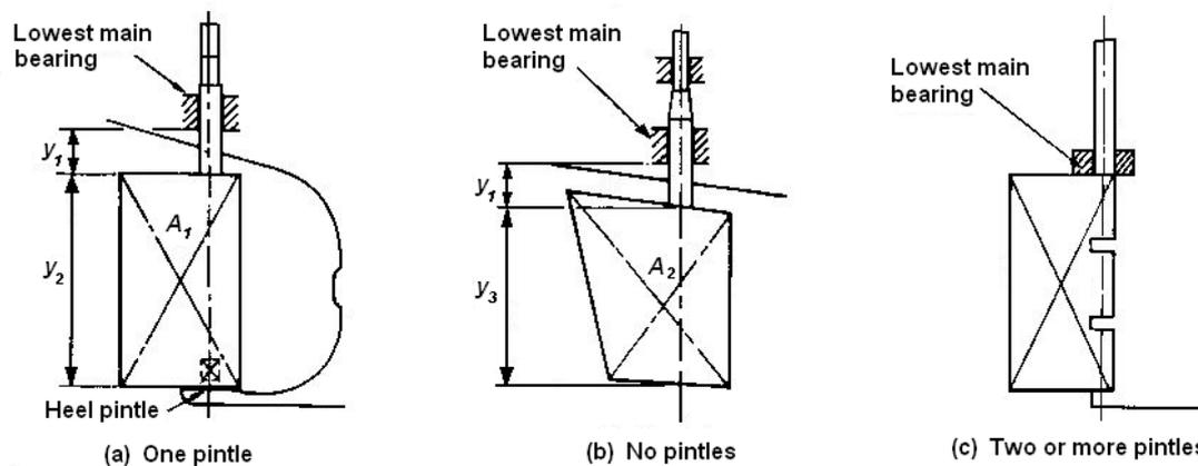
**Fig. 85.** Types of rudder bearing arrangements according to the Lloyd's Register of Shipping [98]
