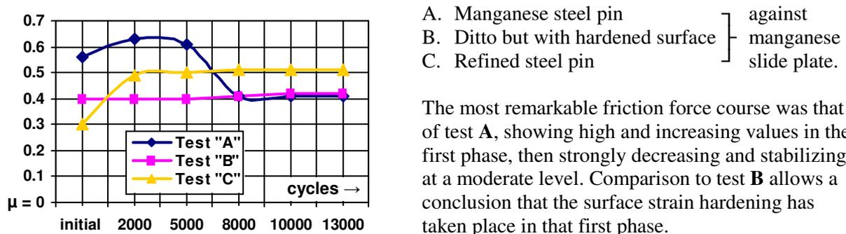
**Fig. 90.** Global variation of friction coefficient during testing
