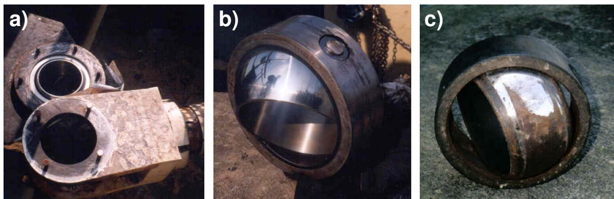
**Fig. 85.** Ineffective lubrication of a cylinder arm ball hinge in gates of the Houtrib Locks in Lelystad
