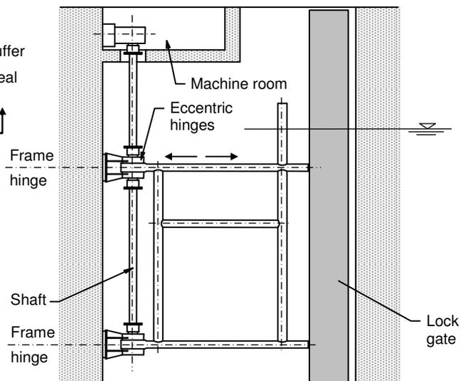
**Fig. 21.** Gate locking frame in the Bergsche Diep Lock near Tholen
