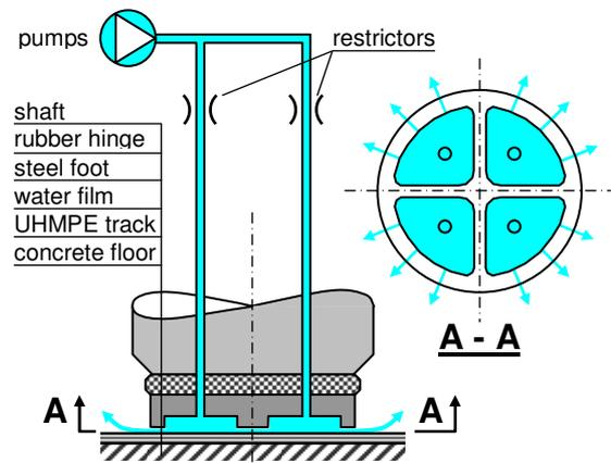
**Fig. 77.** Hydrostatic foot of the New Orange Lock gates in Amsterdam
