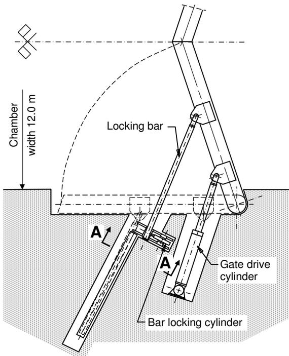
**Fig. 25.** Gate locking in the Merwede Lock in Gorinchem
