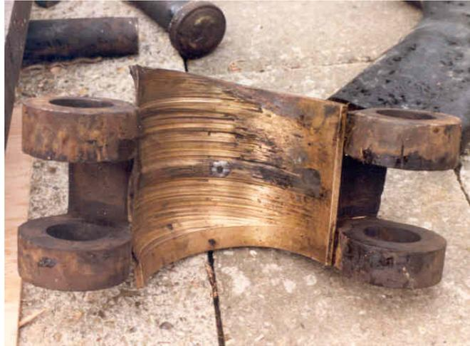
**Fig. 54.** Top hinge collar ring of the old Orange Locks in Amsterdam damaged by wear
