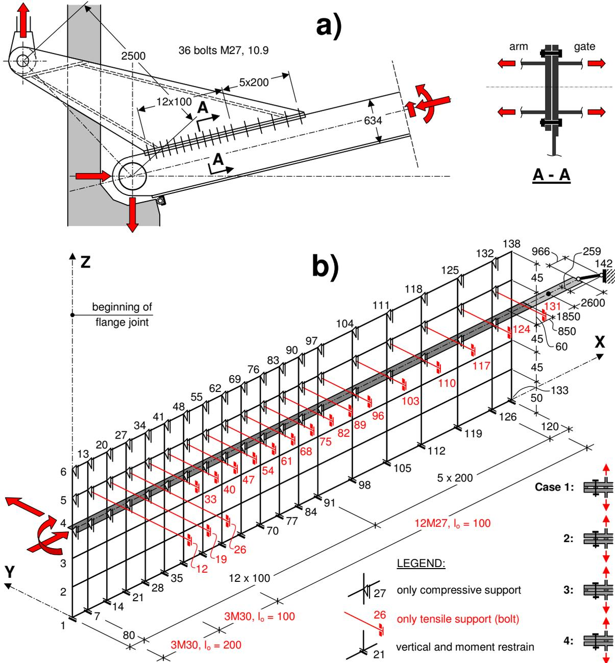
Fig. 72. Orange Locks: drive arm connection (a) and DISCO analysis model for the repair (b) [90]
