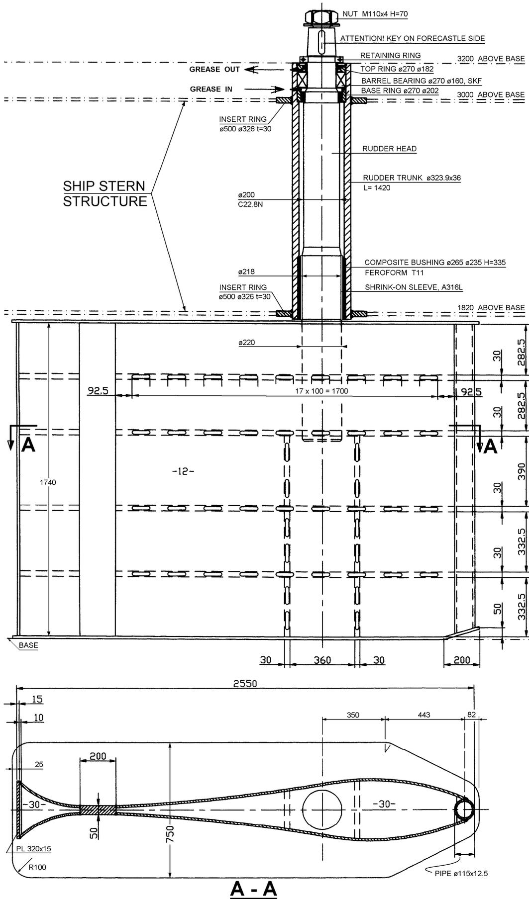
Fig. 84. Ms. JOWI – rudder and its bearings (courtesy Maprom Engineering, Dordrecht)
