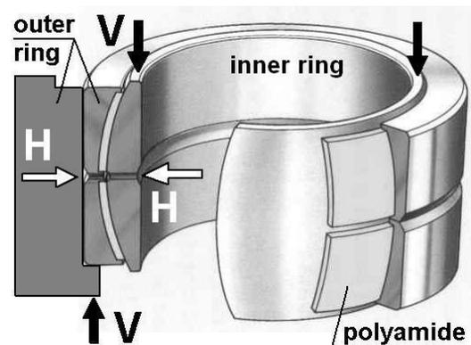
**Fig. 66.** Gate top hinge and the ball bearing of the Orange Locks in Amsterdam
