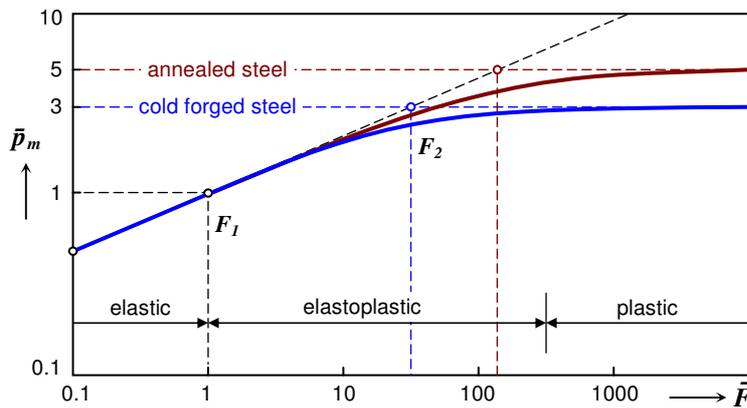
**Fig. 42.** Contact deformation diagram for two groups of steel
