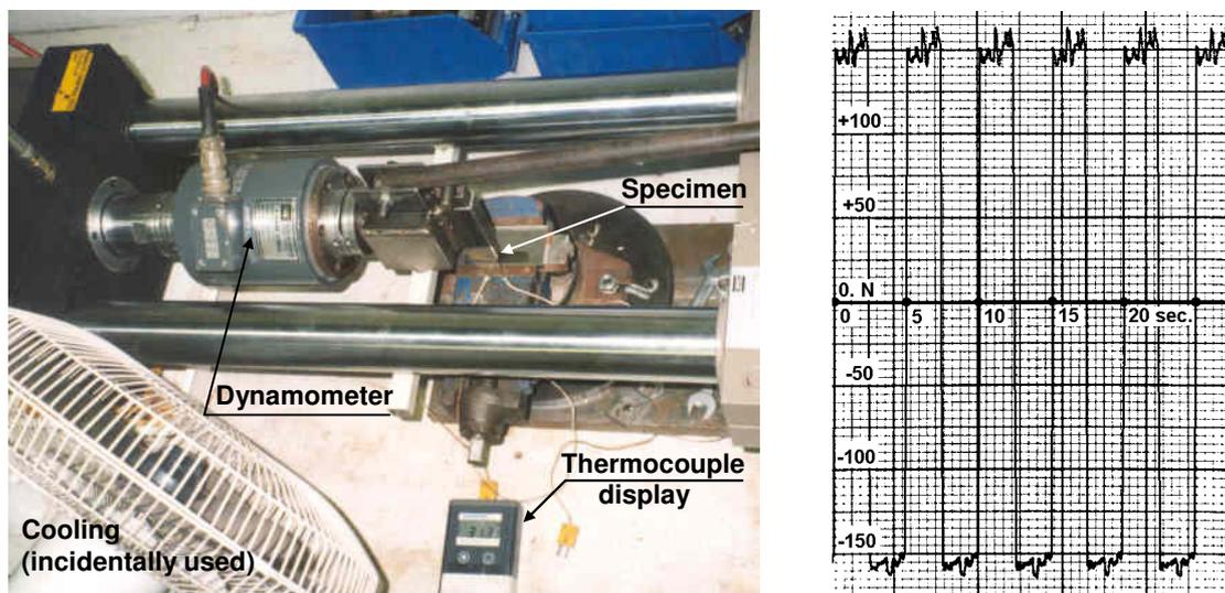
**Fig. 89.** Wear test with friction measurements: left testing table, right friction force record (example)
