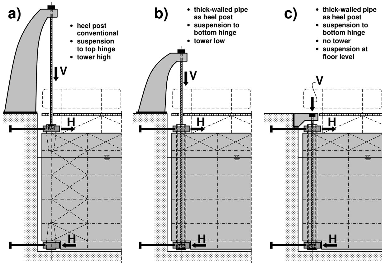
**Fig. 107.** Three basic types of a suspension gate
