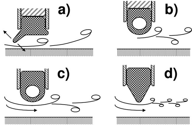
**Fig. 18.** Solution to the vibration problem on the Haringvliet Barrier (**a** → **b**) and on the Hagestein Weir (**c** → **d**)
