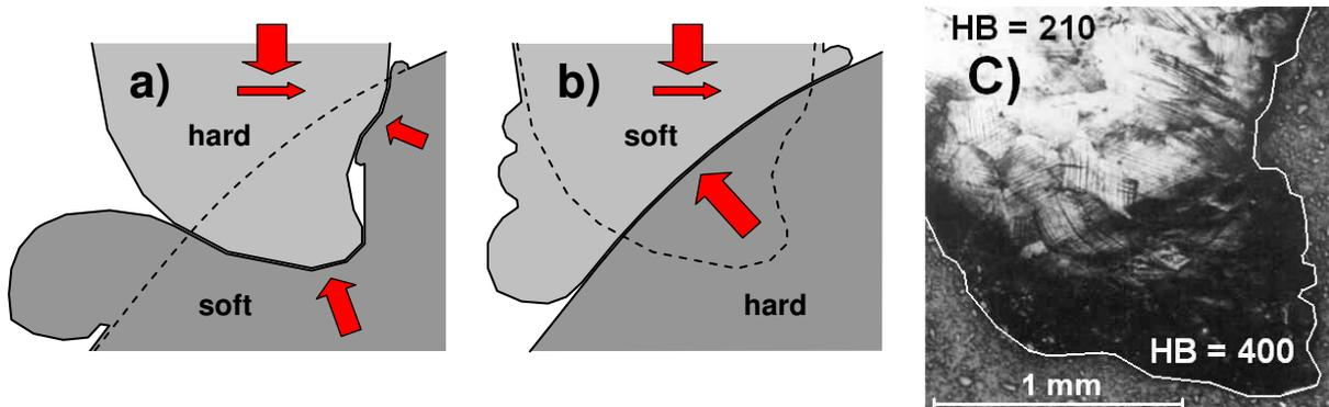
**Fig. 58.** Variants of asperity contact for detail “A” from Fig. 57
