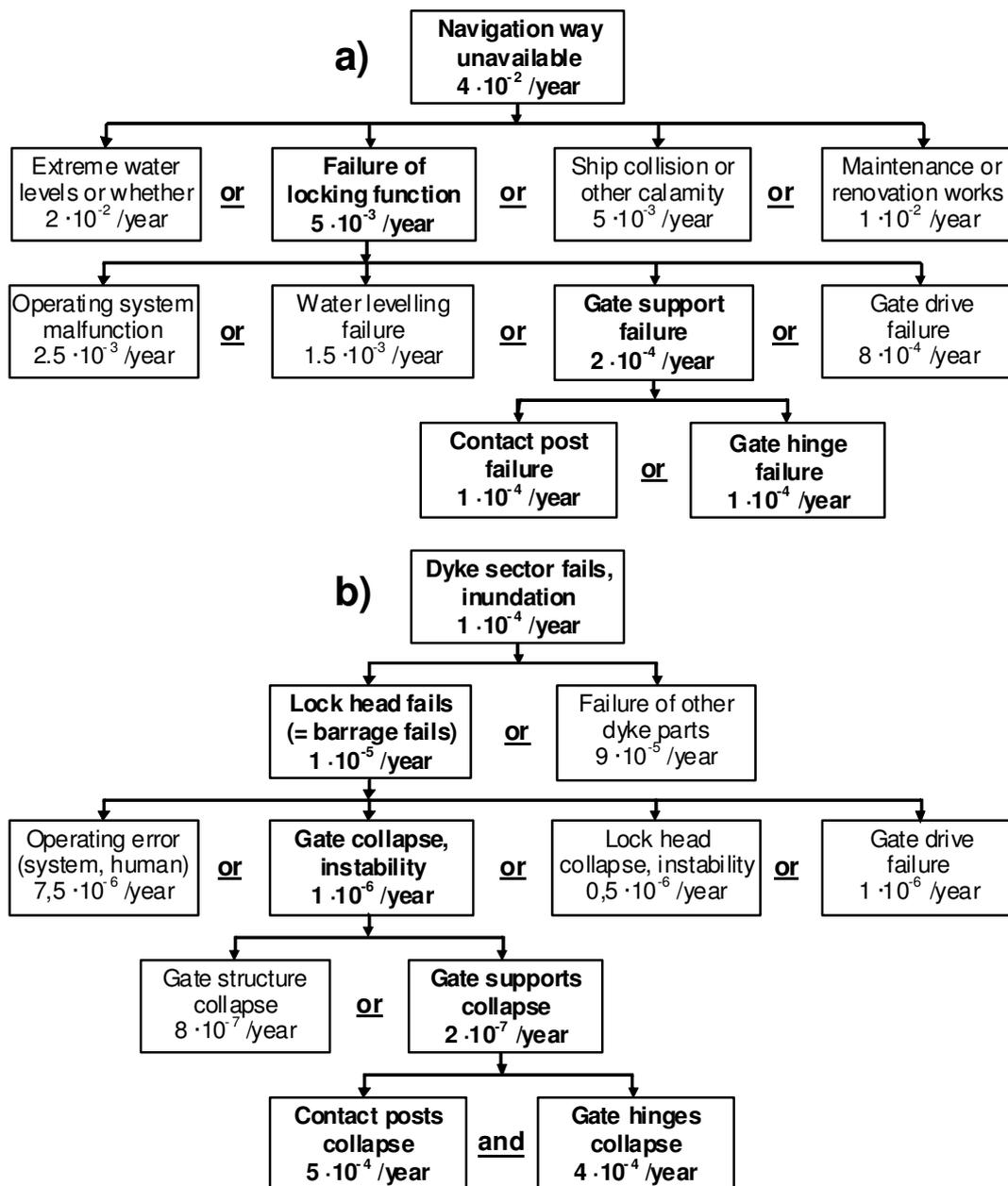
Fig. 8. Fault trees for the navigation (a) and land protection (b) tasks - example
