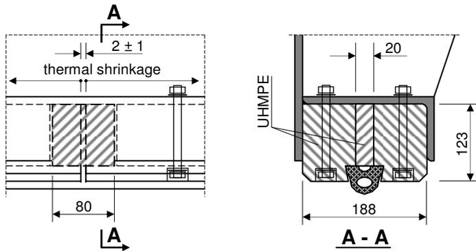
**Fig. 31.** Leak protection for a polyethylene profile joint
