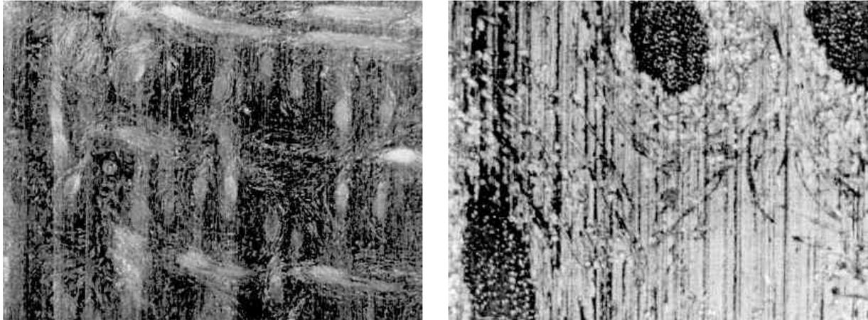
**Fig. 97.** Railko RG2 structure after the wear test, left ~10 x and right ~50 x enlarged, [49]
