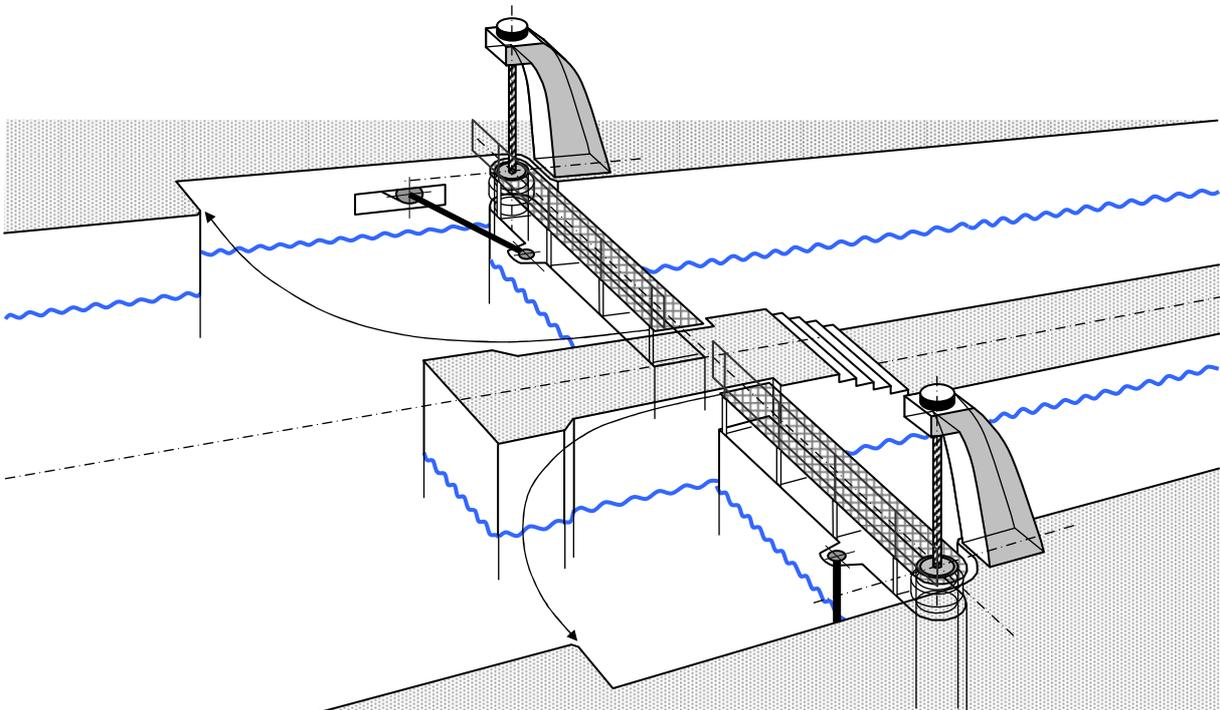
**Fig. 109.** Suspension gate as a single-leaf gate
