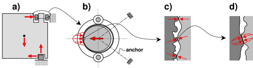
**Fig. 17.** Levels of contact: **a)** system, **b)** component, **c)** segment, **d)** asperity
