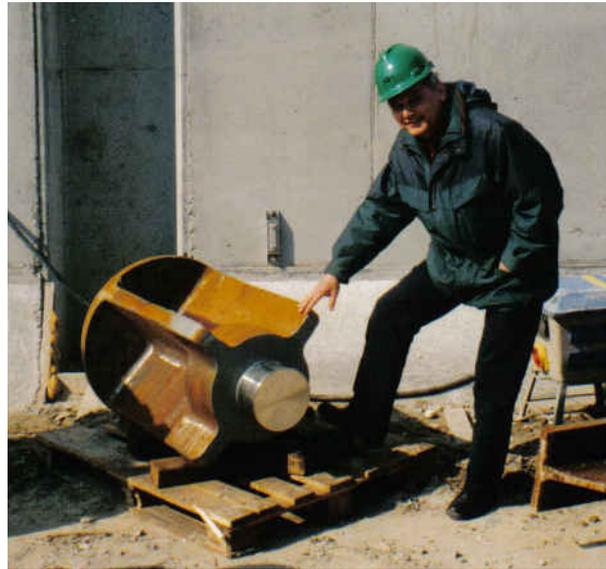
**Fig. 104.** One of the bottom pivots in Naviduct Enkhuizen [43] before installation
