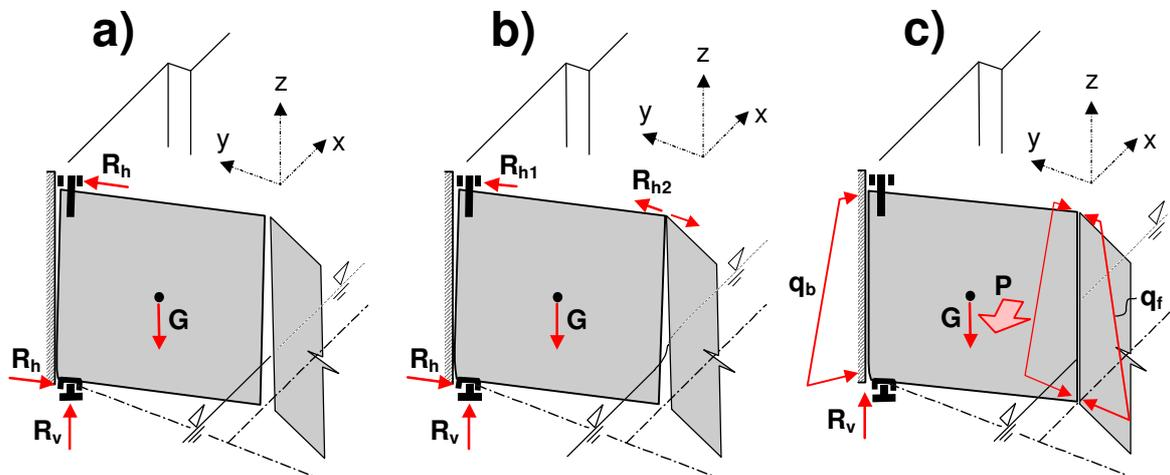
**Fig. 15.** Systems and supporting conditions of a mitre gate during closing
