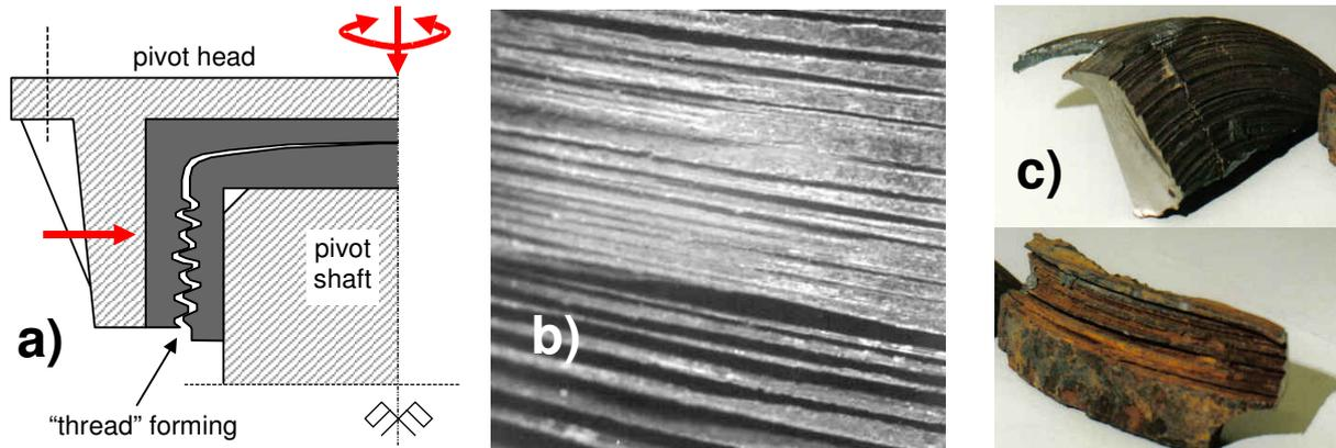
**Fig. 80.** “Thread” forming on a mitre gate bottom pivot:
