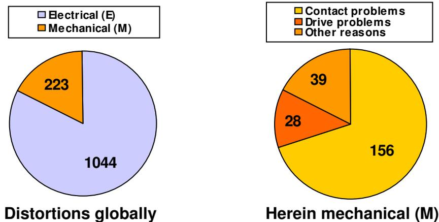
**Fig. 119.** Global pie-charts of hydraulic gate operation distortions on waterways in Limburg
