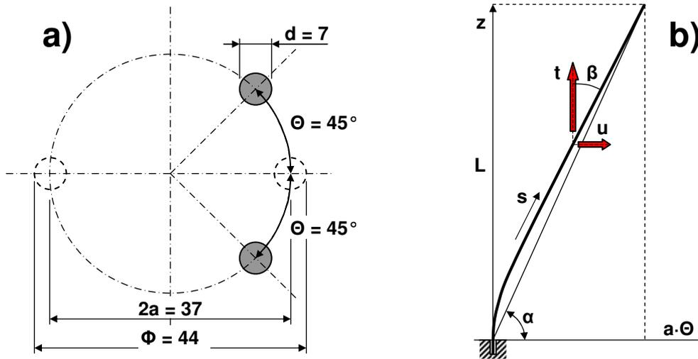
**Fig. 111.** Second-order bending of a wire in the outer layer
