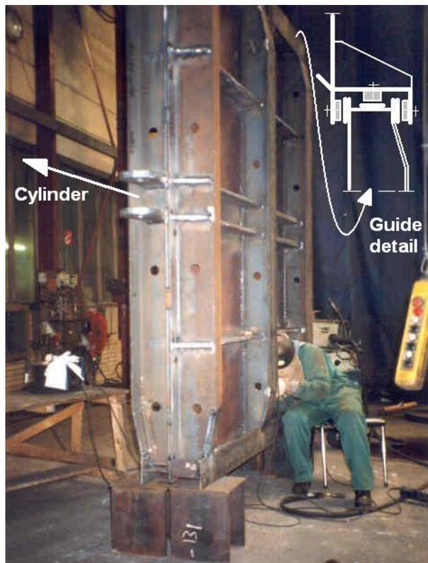
An interesting detail is here that the importance of contact issues has correctly been understood and implied in the manufacturing. Observe that two sluices have been fixed to each other, retaining plates inside. The welding takes now place in the middle of the compound section. The heat input is, there-
