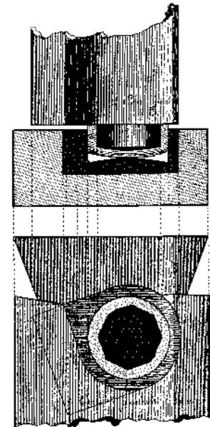
**Fig. 103.** Bottom hinge of an old (XVII century) gate in the Sea Lock in Muiden near Amsterdam [106]
