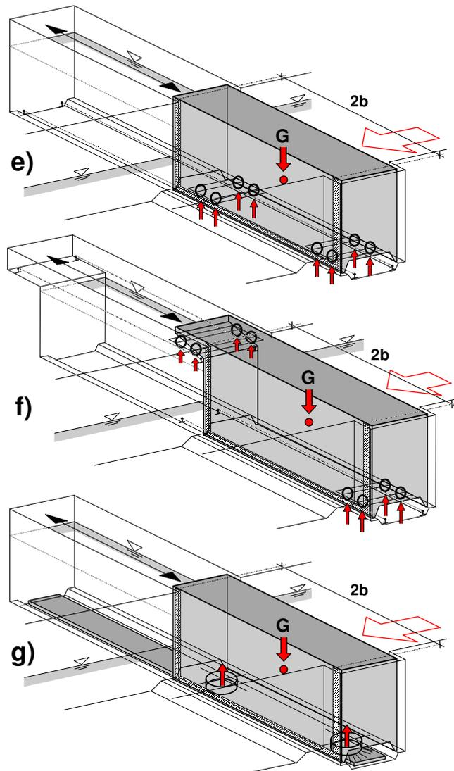
**Fig. 7.** Three rolling gate support systems in regard to vertical loads:
