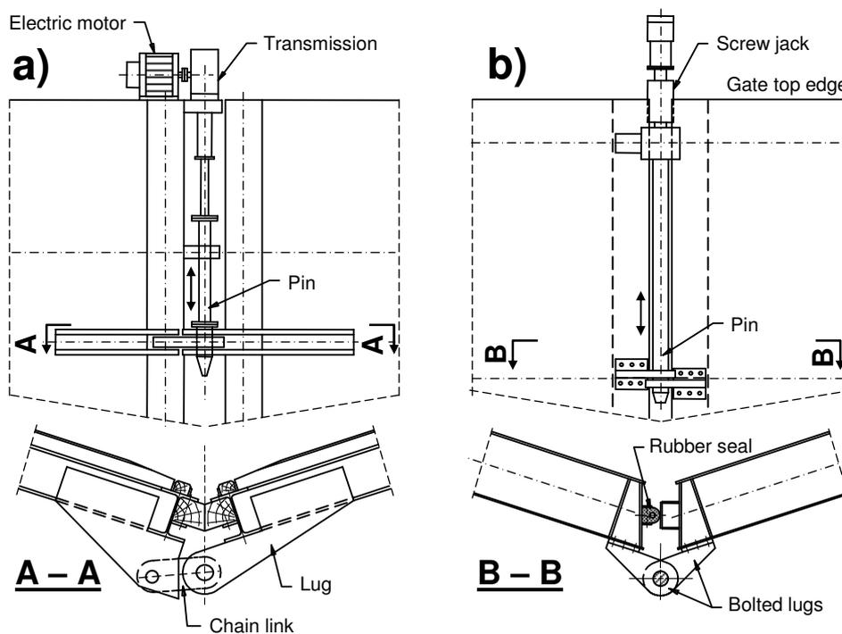
**Fig. 22.** Mitre gate front post locking: **a)** Queens Lock gate in Vreeswijk (present device); **b)** canal locks in Haandrik and Aadorp.
