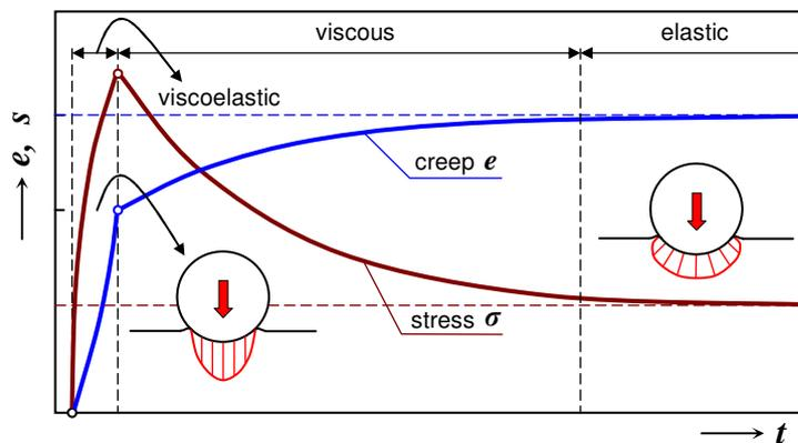
**Fig. 43.** Contact deformation diagram for two groups of steel
