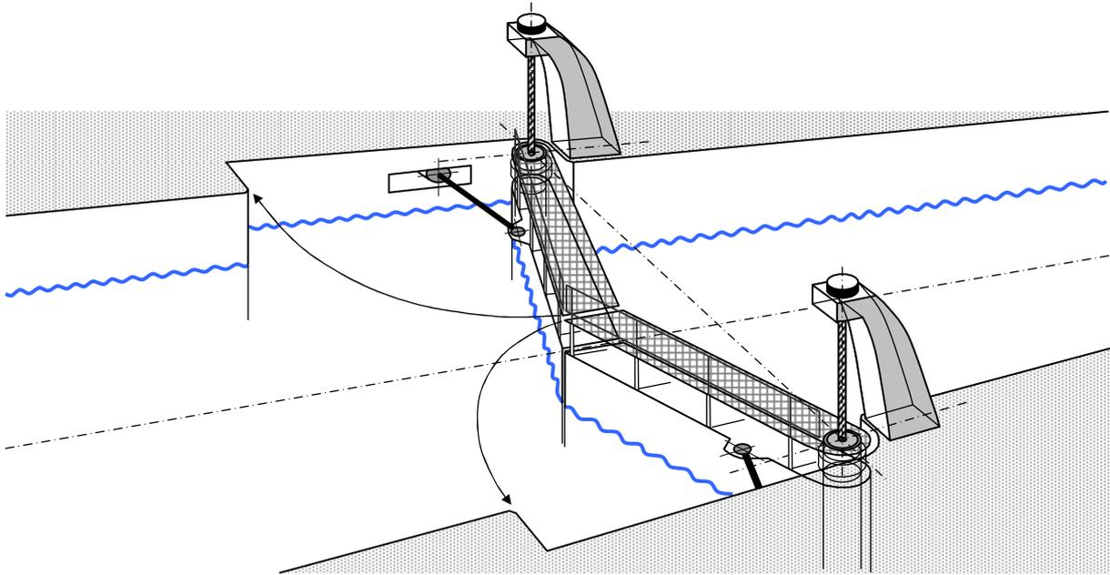
**Fig. 108.** Suspension gate as a mitre gate
