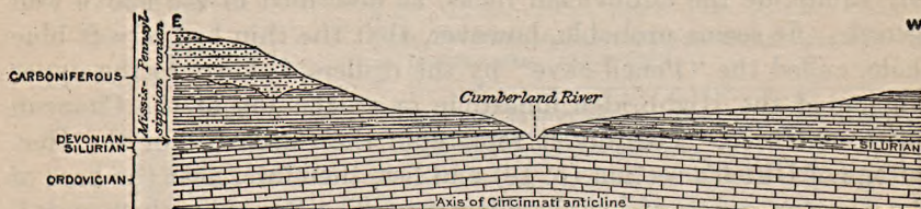
FIGURE 3.—Diagrammatic section from east to west across the axis of the Cincinnati anticline in southern Kentucky, showing supposed stratigraphic position of the Silurian rocks on each side of the axis.
